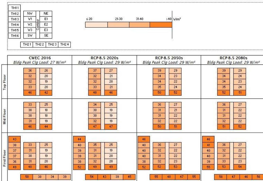
Figure 3.16 Peak cooling load ( $\text{W}/\text{m}^2$ ) at zone level for each climate scenario. A darker shade of orange indicates a higher peak cooling load. Note that the peak cooling load does not account for system efficiency.
