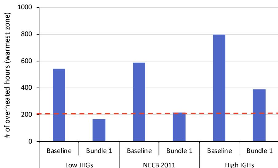
Figure 0.13 Sensitivity analysis of internal heat gains based on new building low rise archetype and Bundle 1, modelled with the RCP-8.5 2050s climate file.
