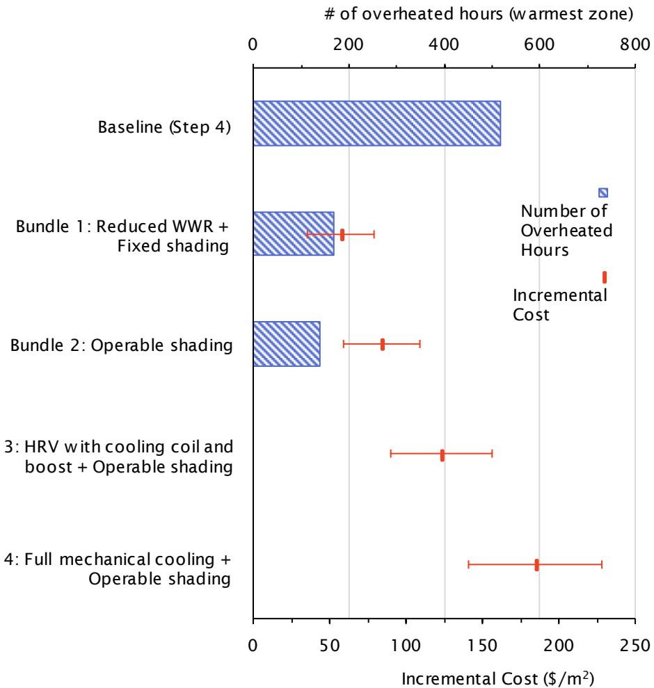
*Figure D.3 Incremental cost (\$/m<sup>2</sup>) for the Step 4 bundles shown together with the number of overheated hours based on RCP-8.5 2050s climate file. The error bars show the high and low incremental bundle cost.*
