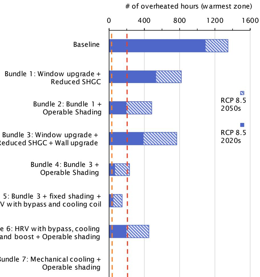
*Figure 3.45 Number of overheated hours for the warmest suite for each modelled bundle. The red dashed line illustrates the 200 hour limit, the orange dashed line illustrates the 20 hour limit for vulnerable population.*
