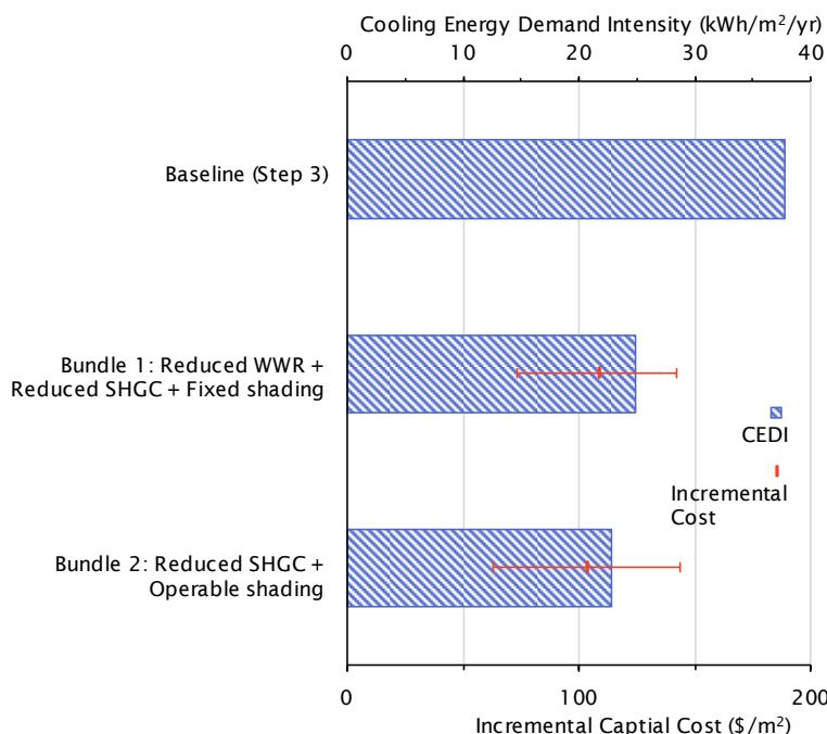
*Figure 3.23 Incremental cost ( $$/m^2$ ) for the Step 3 bundles shown together with the number of overheated hours based on RCP-8.5 2050s climate file. The error bars show the high and low incremental bundle cost.*
