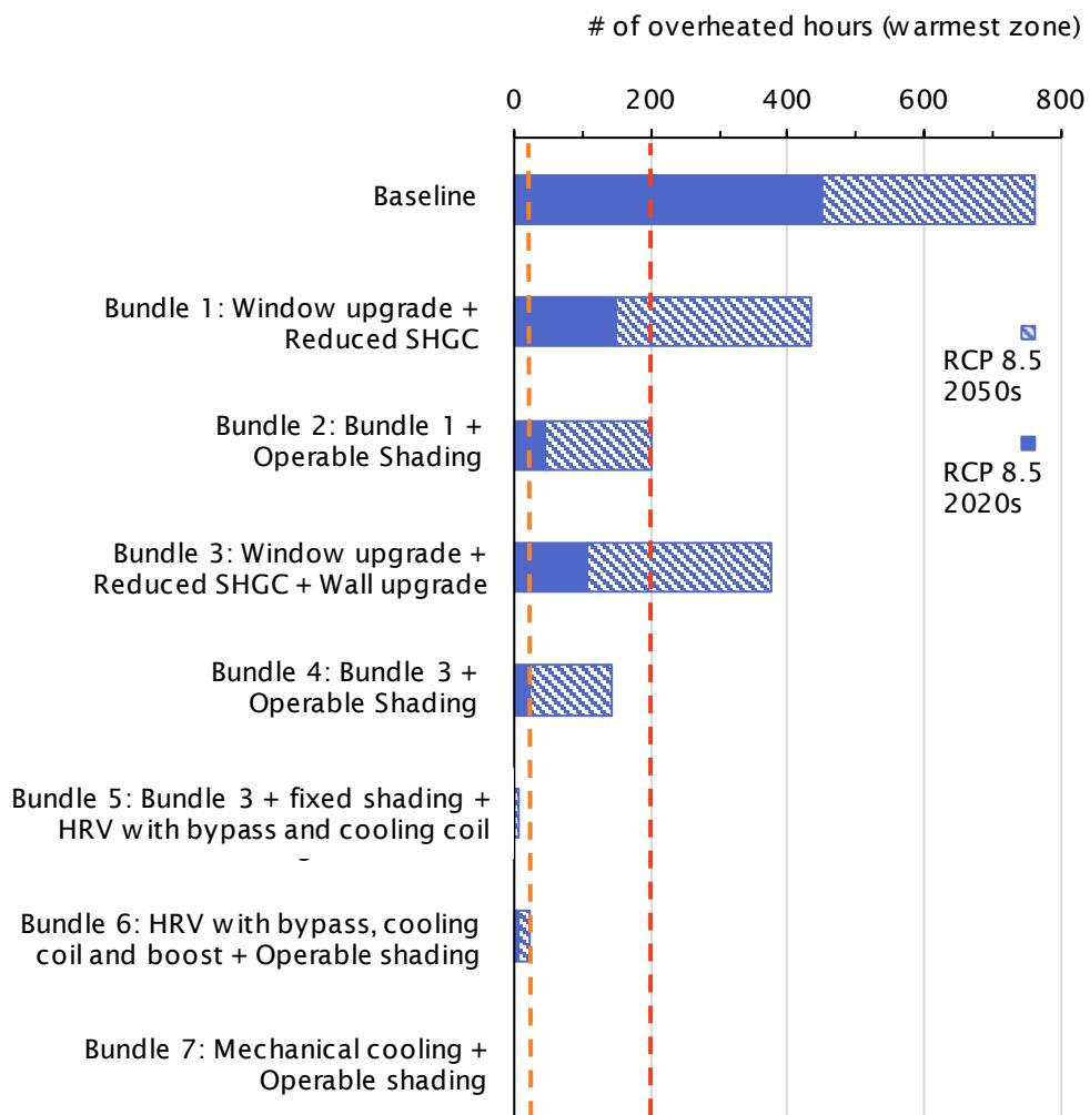
Figure 3.35 Number of overheated hours for the warmest suite for each modelled bundle. The red dashed line illustrates the 200 hour limit, the orange dashed line illustrates the 20 hour limit for vulnerable population.
