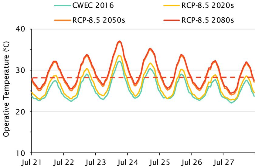
Figure 3.31 Modelled operative temperature (°C) for the warmest suite for the low rise existing building baseline. The interior temperature is shown for the warmest summer week, based on the CWEC 2016, RCP-8.5 2020s, 2050s and 2080s climate files. The red dashed line illustrates the 80% acceptability limit based on the CWEC 2016 climate file.
