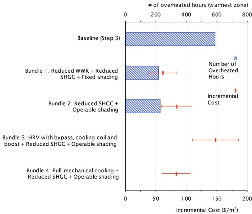
Figure 0.1 Incremental cost (\$/m<sup>2</sup>) for the Step 3 bundles shown together with the number of overheated hours based on RCP-8.5 2050s climate file. The error bars show the high and low incremental bundle cost.
