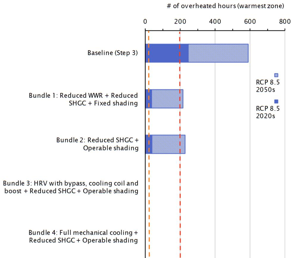
*Figure 3.7 Number of overheated hours for the warmest zone in the Step 3 low rise new building baseline and bundle archetypes, based on the RCP-8.5 2020s and 2050s climate files. The red dashed line illustrates the 200 hour limit, and the orange dashed line illustrates the 20 hour limit for vulnerable population.*
