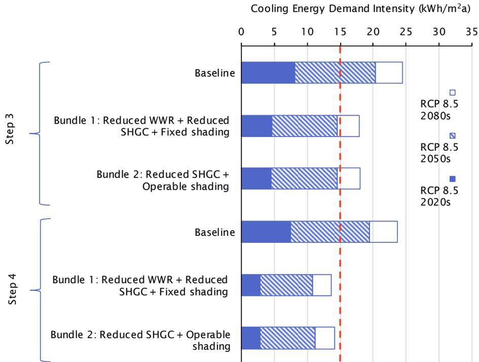
Figure 4.5 Cooling energy demand intensity (CEDI) for new high rise at building level, modelled with the RCP-8.5 2020s, 2050s, and 2080s climate files. The red dashed line illustrates the PHI limit of 15 kWh/m<sup>2</sup>a.
