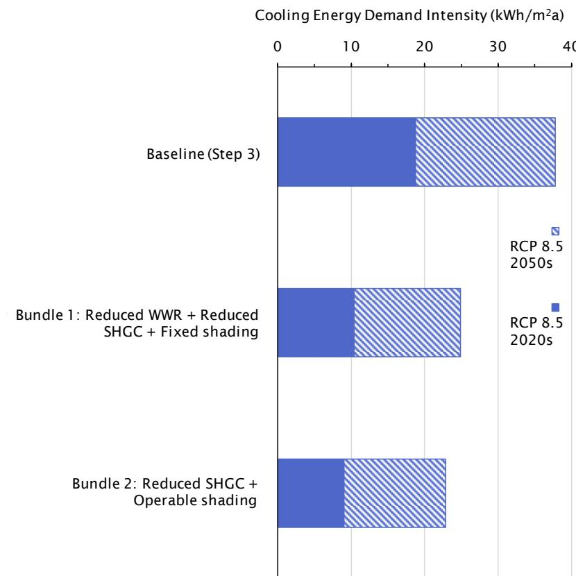
*Figure 3.21 Cooling energy demand intensity (kWh/m<sup>2</sup>a) for the warmest suite for the Step 3 baseline and modelled bundles, for RCP-8.5 2020s and 2050s climate files.*
