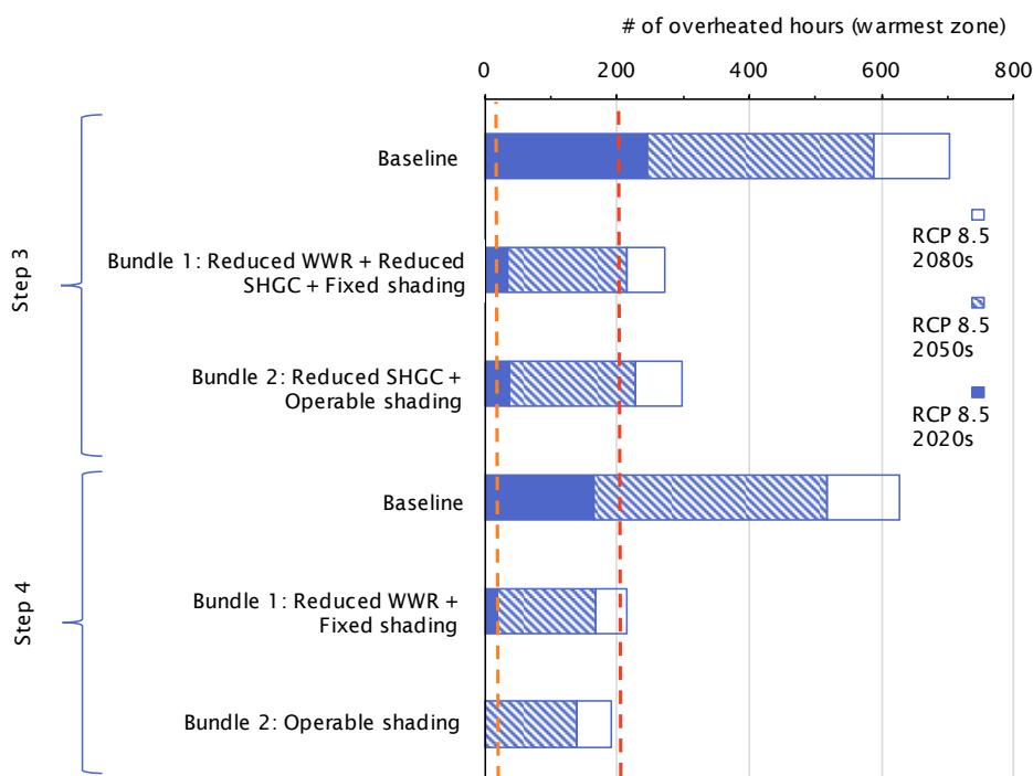
*Figure 4.4 Number of overheated hours for the warmest zone, modelled with the RCP-8.5 2020s, 2050s, and 2080s climate files. The red dashed line illustrates the 200 hour threshold, and the orange dashed line illustrates the 20 hour threshold for vulnerable populations.*
