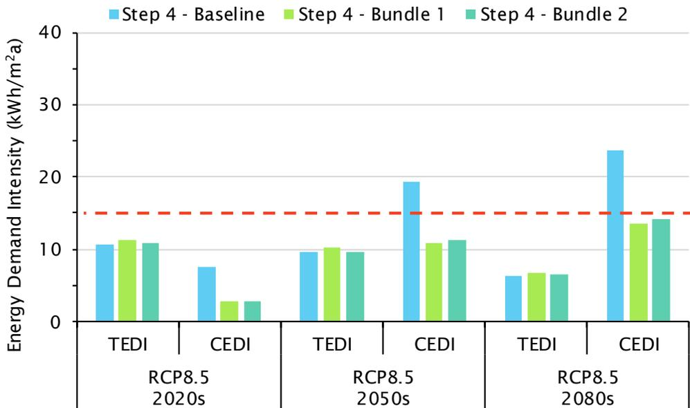
Figure 3.26 TEDI and CEDI results for the Step 4 high rise new building baseline and bundle archetypes based on CWEC 2016, RCP-8.5 2020s, 2050s, and 2080s climate files. The red dashed line illustrates the Step 4 TEDI target (15 kWh/m<sup>2</sup>a), and reference CEDI target (15 kWh/m<sup>2</sup>a)
