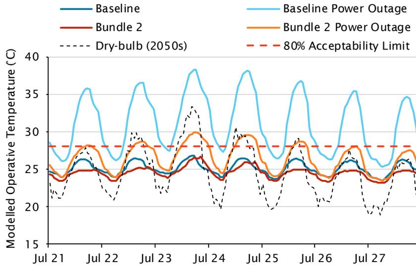
Figure 0.15 Modelled operative temperature for the Step 4 high rise new building baseline and Bundle 2, during normal operation and during a power outage event for a summer week.
