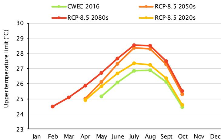
Figure 2.1 The upper 80% acceptability temperature limit for each month following ASHRAE 55-2010 Section 5.3, for the CWEC 2016, RCP-8.5 2020s, 2050s and 2080s climate files for UBC.
