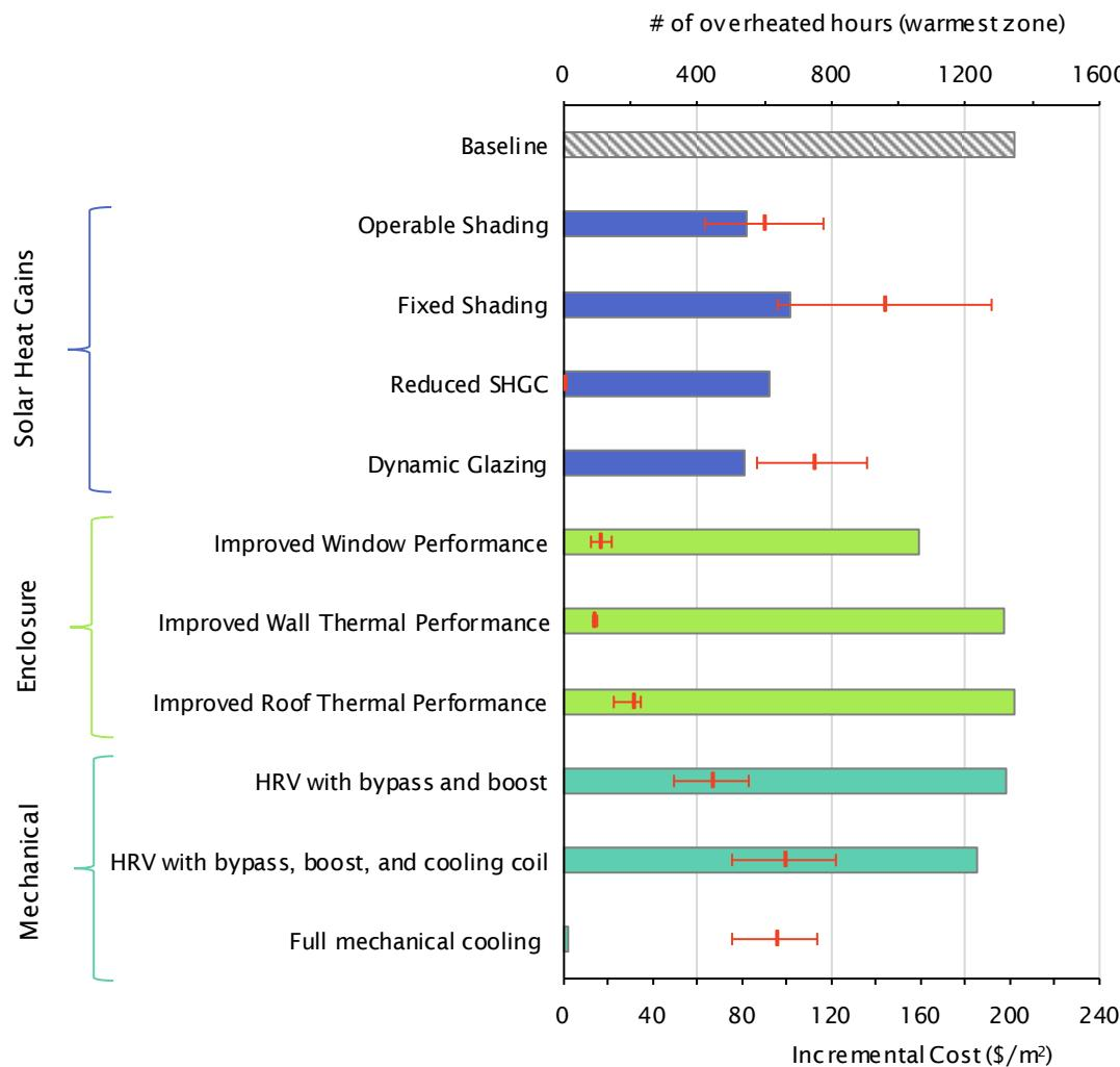
Figure 3.44 The red lines show the incremental cost (\$/m<sup>2</sup>) on building level, the error bars show the high and low cost. The number of overheated hours is shown for the warmest suite based on RCP-8.5 2050s climate file.
