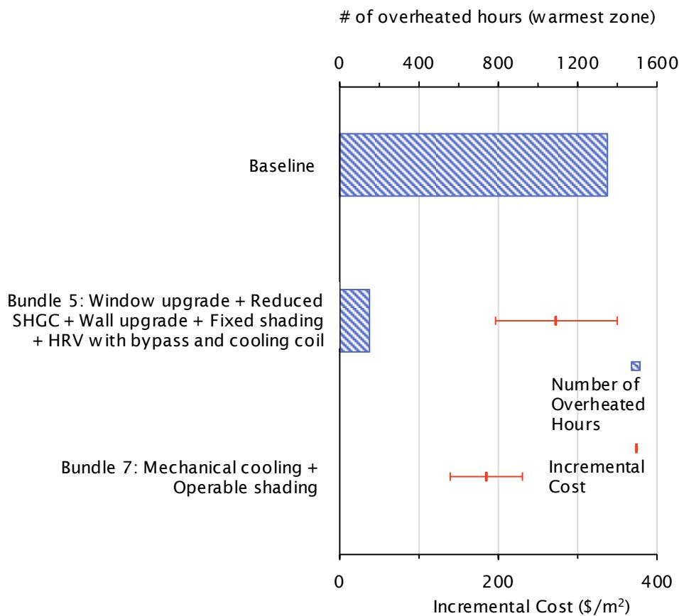
*Figure 3.47 Incremental cost (\$/m<sup>2</sup>) for the bundles shown together with the number of overheated hours based on RCP-8.5 2050s climate file. The error bars show the high and low incremental bundle cost.*
