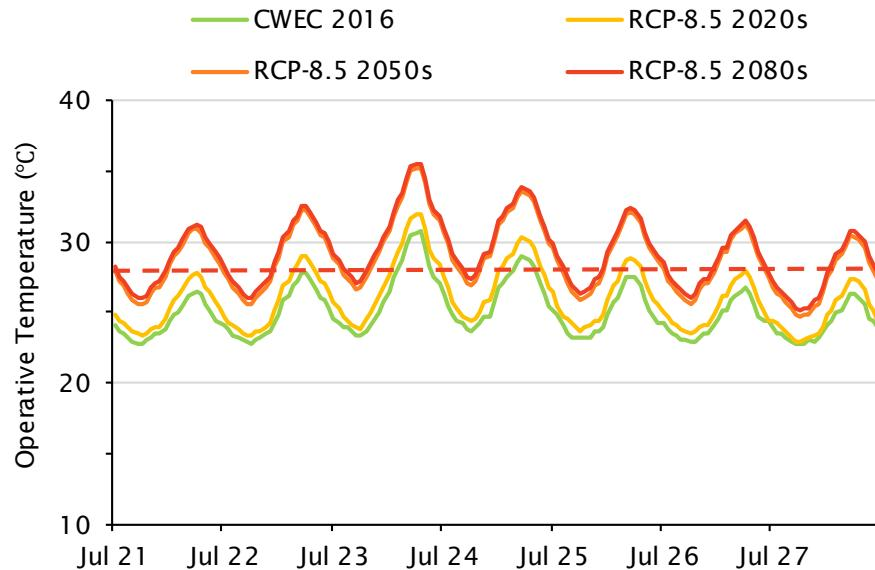
Figure 3.3 Modelled interior operative temperature (°C) for the warmest suite for the low rise new building baseline, shown for one summer week, based on the CWEC 2016, RCP-8.5 2020s, 2050s and 2080s climate files. The red dashed line illustrates the 80% acceptability limit based on the CWEC 2016 climate file.
