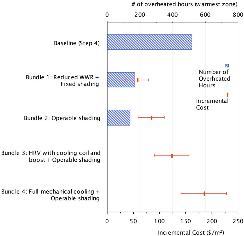
Figure D.3 Incremental cost (\$/m<sup>2</sup>) for the Step 4 bundles shown together with the number of overheated hours based on RCP-8.5 2050s climate file. The error bars show the high and low incremental bundle cost.
