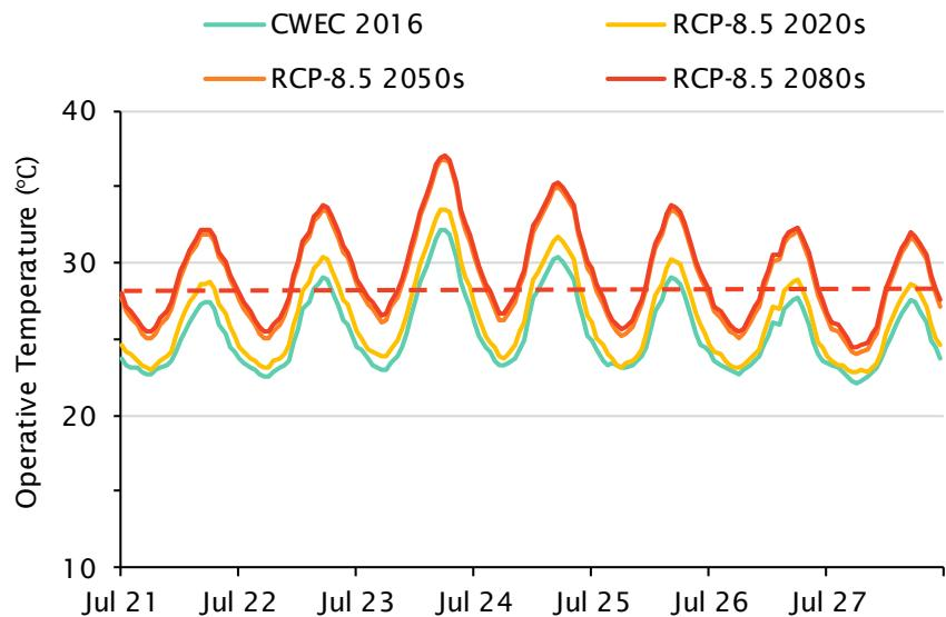
Figure 3.31 shows the modelled hourly operative temperature for the warmest suite during the warmest week for the low rise existing building baseline. The operative temperature is shown based on the CWEC 2016 climate file and RCP-8.5 2020s, 2050s and 2080s. The red dashed line illustrates the 80% acceptability limit based on the CWEC 2016 file.
