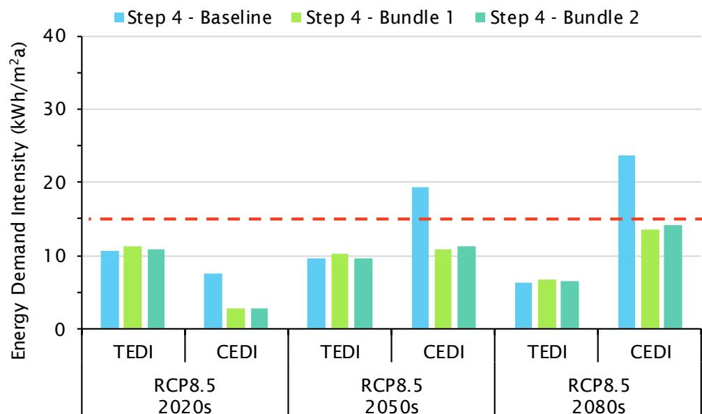
Figure 3.26 TEDI and CEDI results for the Step 4 high rise new building baseline and bundle archetypes based on CWEC 2016, RCP-8.5 2020s, 2050s, and 2080s climate files. The red dashed line illustrates the Step 4 TEDI target (15 kWh/m<sup>2</sup>a), and reference CEDI target (15 kWh/m<sup>2</sup>a)
