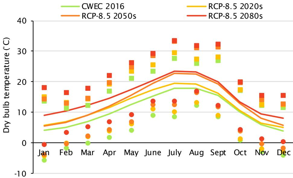
Figure 2.2 Monthly average, maximum, and minimum dry-bulb temperature (°C) for CWEC 2016 and RCP-8.5 2020s, 2050s, and 2080s climate files for UBC.
