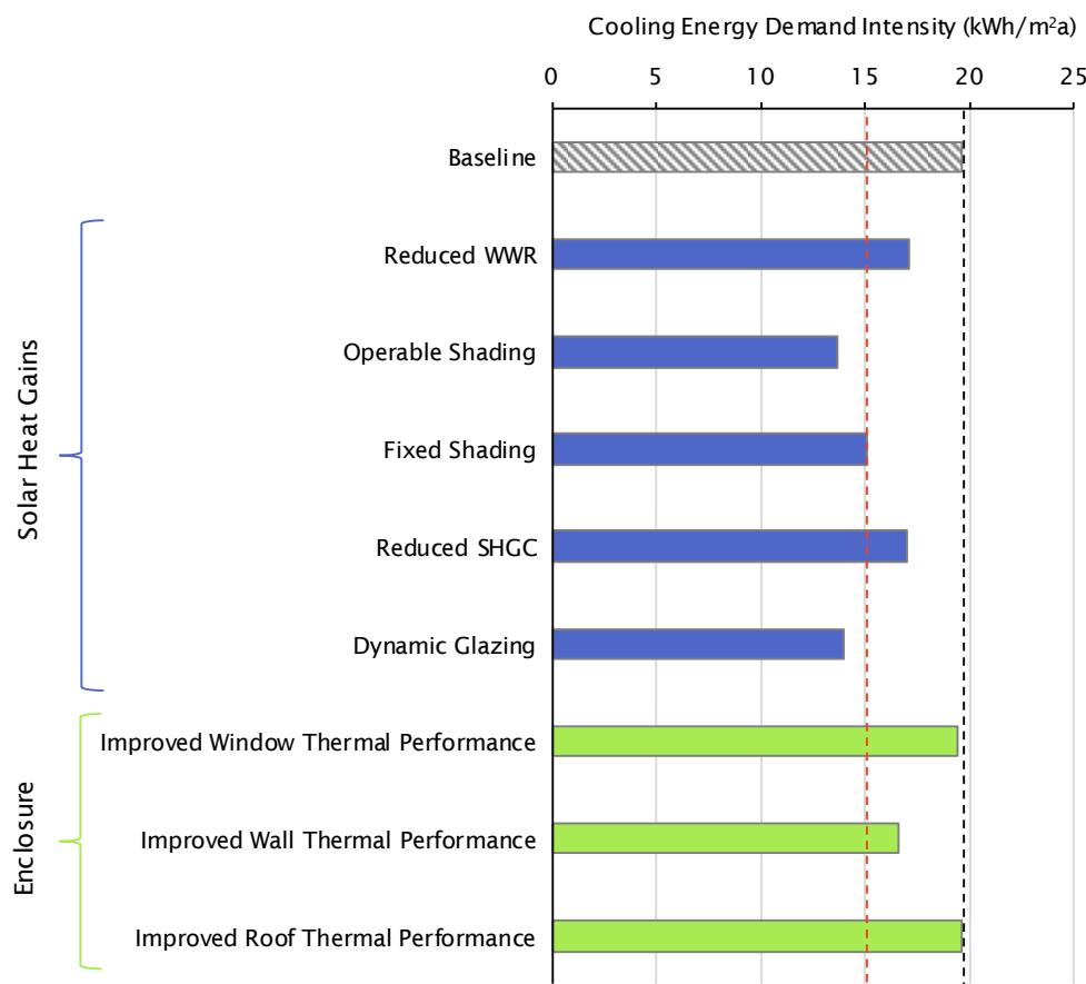
*Figure 3.18 Building annual cooling energy demand intensity for the high rise new building baseline archetype and individual climate adaptation measures, modelled with the RCP-8.5 2050s climate file. The red dashed line indicates for the PHI cooling energy demand criteria (15 kWh/m<sup>2</sup>a), and the black dashed line presents the baseline results.*
