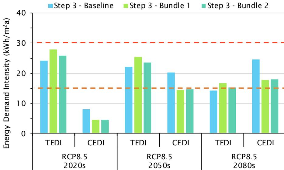
Figure 3.22 TEDI and CEDI results for the Step 3 high rise new building baseline and bundle archetypes based on RCP-8.5 2020s, 2050s, and 2080s climate files. The red dashed line illustrates the Step 3 TEDI target (30 kWh/m²a), and the orange dashed line illustrates a theoretical reference CEDI target (15 kWh/m²a)
