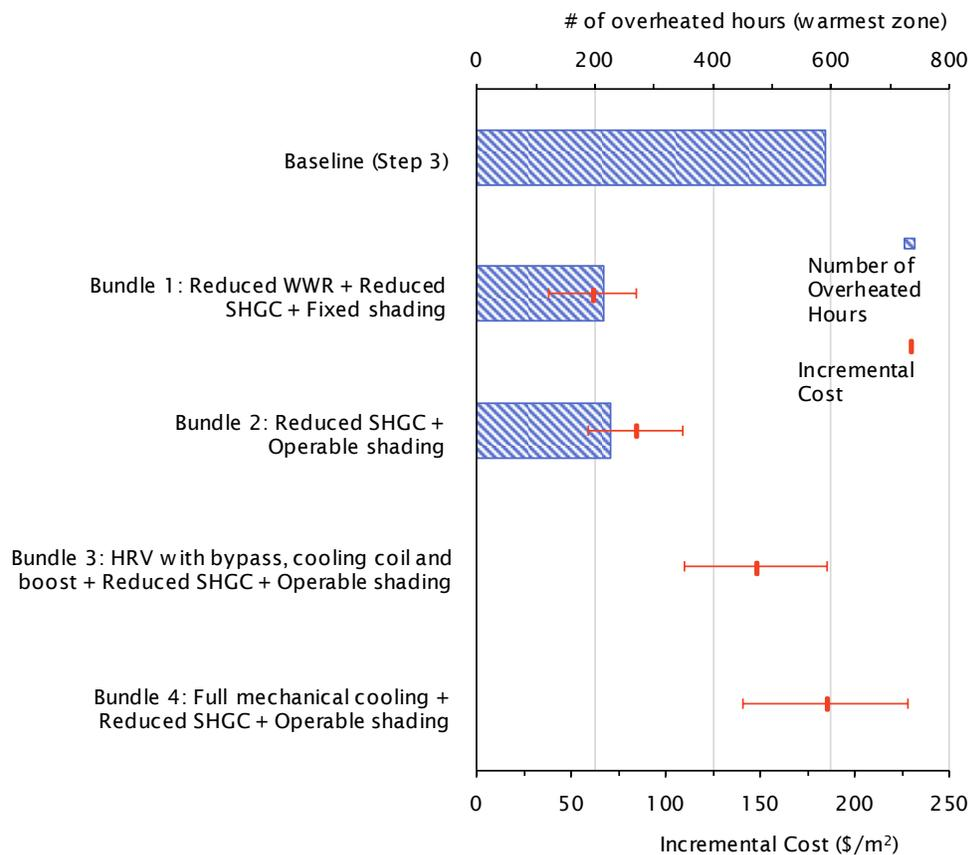
Figure D.1 Incremental cost (\$/m<sup>2</sup>) for the Step 3 bundles shown together with the number of overheated hours based on RCP-8.5 2050s climate file. The error bars show the high and low incremental bundle cost.
