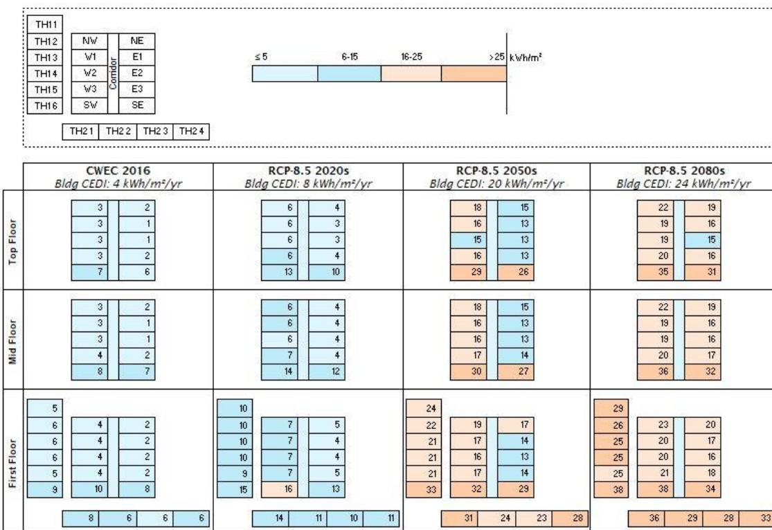
**Figure 3.15 Cooling energy demand intensity ( $\text{kWh}/\text{m}^2\text{a}$ ) at zone level for each climate file.**
