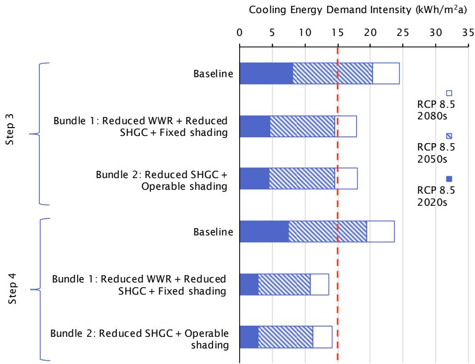
*Figure 0.17 Cooling energy demand intensity (CEDI) for new high rise at building level, modelled with the RCP-8.5 2020s, 2050s, and 2080s climate files. The red dashed line illustrates the PHI limit of 15 kWh/m<sup>2</sup>a.*
