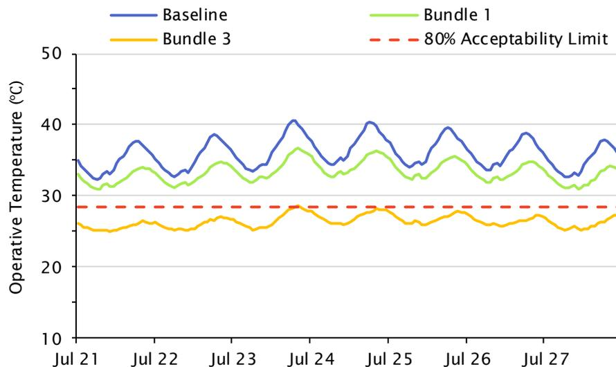
Figure 4.2 Modelled operative temperature for low rise new building Step 3 baseline, bundle 1 and bundle 3 in the event of no natural ventilation, based on the RCP-8.5 2050s climate file. The indoor temperatures are shown together with dry-bulb outdoor temperature for a summer week. The red dashed line illustrates the 80% acceptability limit.
