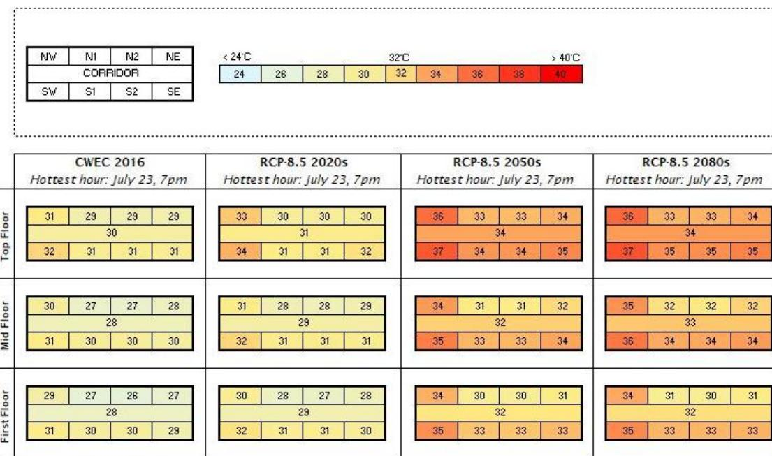
*Figure 3.30 Modelled peak operative temperature (°C) for each zone and climate file. The zones are colour coded to illustrate the variation in peak temperature. A darker shade of red indicates a higher modelled peak temperature.*
