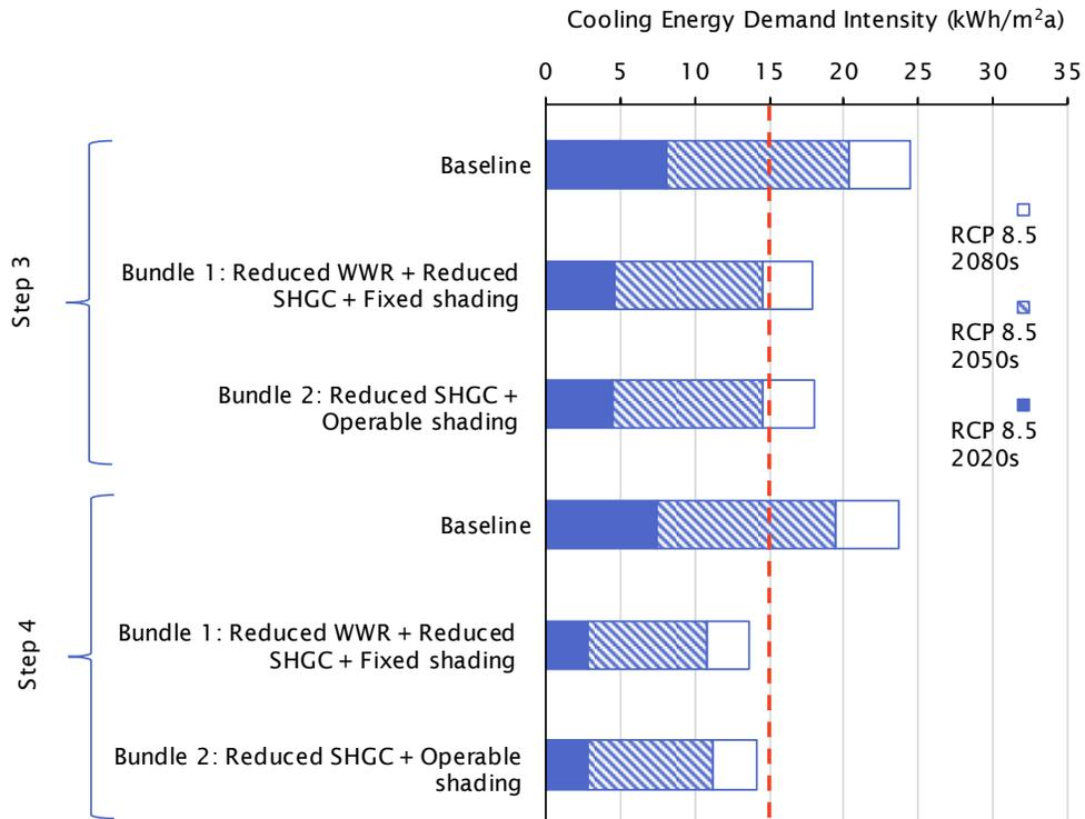
Figure 0.17 Cooling energy demand intensity (CEDI) for new high rise at building level, modelled with the RCP-8.5 2020s, 2050s, and 2080s climate files. The red dashed line illustrates the PHI limit of 15 kWh/m<sup>2</sup>a.
