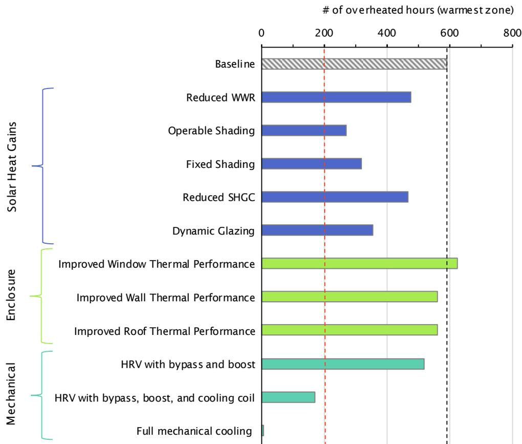
Figure 3.5. Number of overheated hours for the warmest zone for the baseline and each individual CAMM, modelled with the RCP-8.5 2050s climate file. The red dashed line illustrates the 200 hour limit, and the black dashed line indicates the baseline results.
