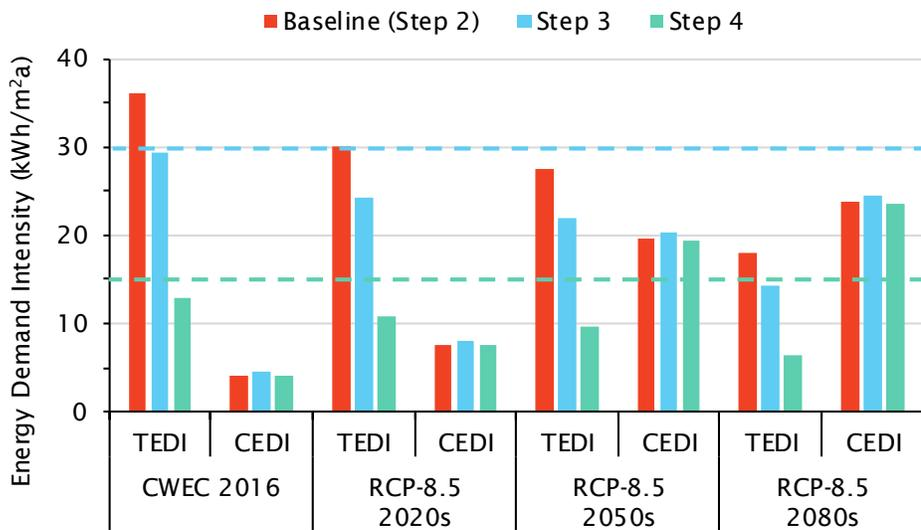
Figure 3.20 TEDI and CEDI for the baseline (Step 2) archetype and bundle baselines (Step 3 and Step 4), the blue and green dashed line show the TEDI target for Step 3 (30 kWh/m²a) and Step 4 (15 kWh/m²a), respectively.
