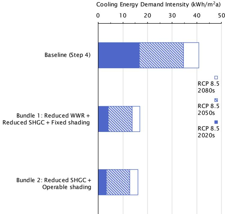
Figure 3.25 Cooling energy demand intensity (kWh/m²a) for the warmest suite for the Step 4 baseline and modelled bundles, modelled with RCP-8.5 2020s and 2050s climate files
