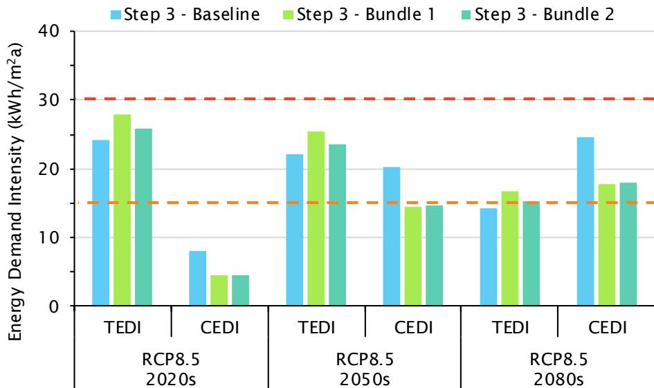
Figure 3.22 TEDI and CEDI results for the Step 3 high rise new building baseline and bundle archetypes based on RCP-8.5 2020s, 2050s, and 2080s climate files. The red dashed line illustrates the Step 3 TEDI target (30 kWh/m<sup>2</sup>a), and the orange dashed line illustrates a theoretical reference CEDI target (15 kWh/m<sup>2</sup>a)
