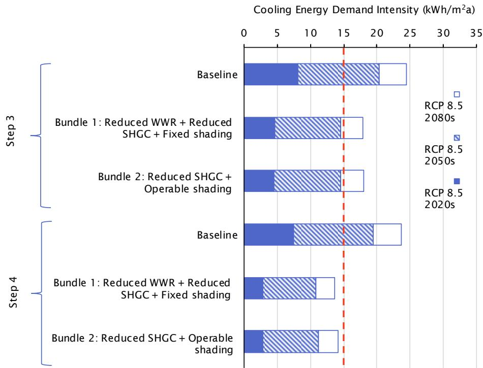
Figure 4.5 Cooling energy demand intensity (CEDI) for new high rise at building level, modelled with the RCP-8.5 2020s, 2050s, and 2080s climate files. The red dashed line illustrates the PHI limit of 15 kWh/m<sup>2</sup>a.
