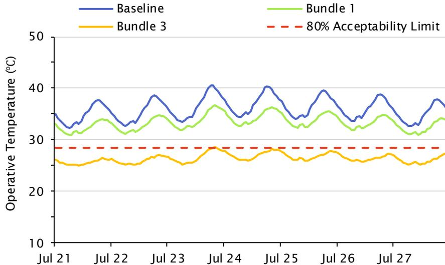
Figure 0.14 Modelled operative temperature for low rise new building Step 3 baseline, bundle 1 and bundle 3 in the event of no natural ventilation, based on the RCP-8.5 2050s climate file. The indoor temperatures are shown together with dry-bulb outdoor temperature for a summer week. The red dashed line illustrates the 80% acceptability limit.
