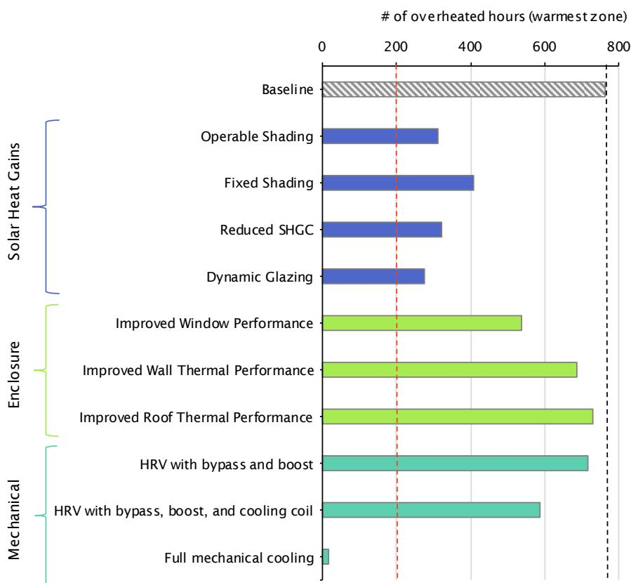
*Figure 3.33 Number of overheated hours for the warmest zone and each individual climate adaptation measure, modelled with the RCP-8.5 2050s climate file. The red dashed line illustrates the 200 hour limit, and the black dashed line presents the baseline results.*
