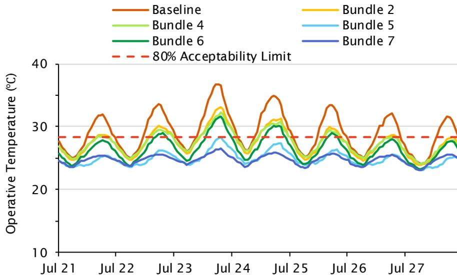
Figure 3.36 Modelled operative temperature (°C) for the warmest suite for the low rise existing building baseline and bundles based on the RCP-8.5 2050s climate file, shown for the hottest summer week.
