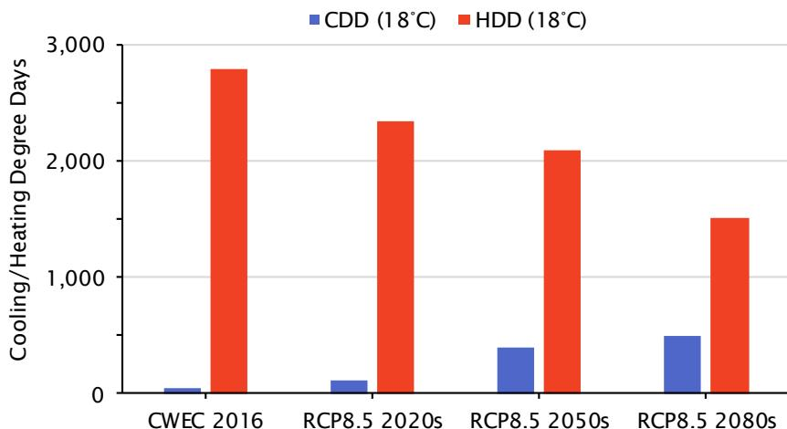
Figure 2.3 Cooling and heating degree days based on the CWEC 2016 file and RCP-8.5 2020s, 2050s and 2080s for UBC.
