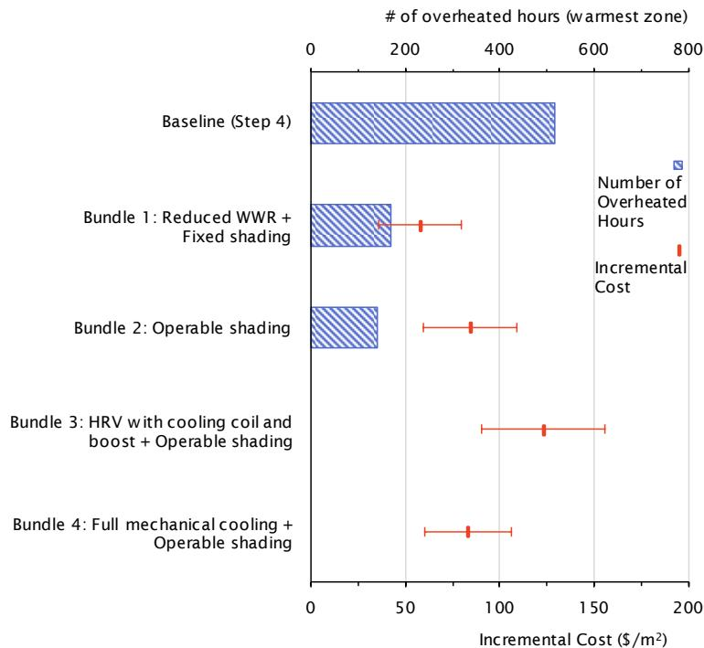
*Figure 0.2 Incremental cost (\$/m<sup>2</sup>) for the Step 4 bundles shown together with the number of overheated hours based on RCP-8.5 2050s climate file. The error bars show the high and low incremental bundle cost.*
