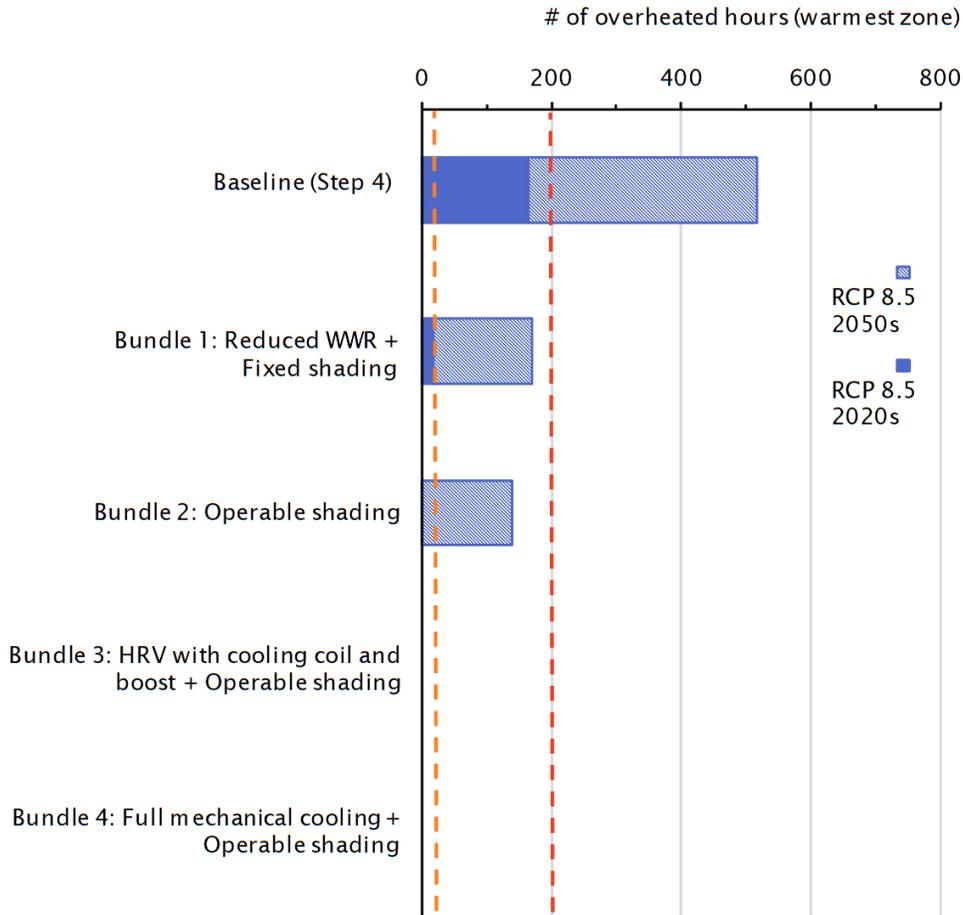
Figure 3.11 Number of overheated hours for the Step 4 low rise new building baseline and modelled bundles based on the RCP-8.5 2020s and 2050s climate files. The red dashed line illustrates the 200 hour limit, and the orange dashed line illustrates the 20 hour limit for vulnerable population.
