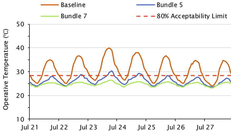
Figure 3.46 Modelled operative temperature (°C) for the warmest suite for the high rise existing building baseline and bundles based on the RCP-8.5 2050s climate file, shown for one summer week.
