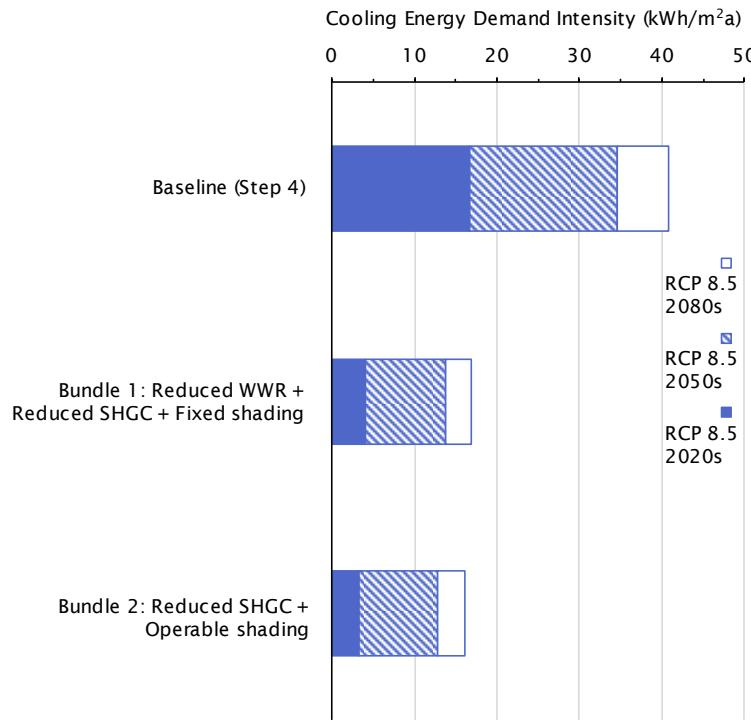
*Figure 3.25 Cooling energy demand intensity (kWh/m<sup>2</sup>a) for the warmest suite for the Step 4 baseline and modelled bundles, modelled with RCP-8.5 2020s and 2050s climate files*
