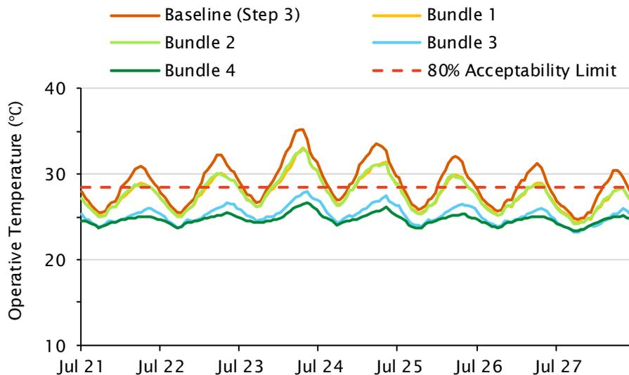
Figure 3.8 Modelled operative temperature (°C) for the warmest suite for the Step 3 low rise new building baseline and bundles based on the RCP-8.5 2050s climate file, shown for the hottest summer week.
