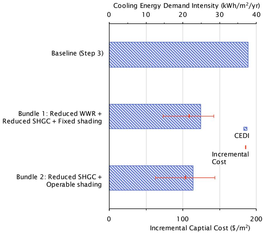
Figure 0.5 Incremental cost (\$/m<sup>2</sup>) for the Step 3 high rise bundles shown together with the number of overheated hours based on RCP-8.5 2050s climate file. The error bars show the high and low incremental bundle cost.
