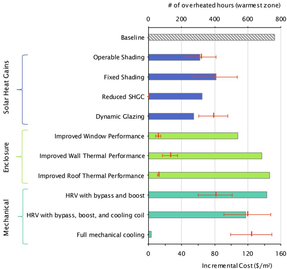
Figure 3.34 The red lines show the incremental cost (\$/m<sup>2</sup>) on building level, the error bars show the high and low cost. The number of overheated hours is shown for the warmest suite based on RCP-8.5 2050s climate file.
