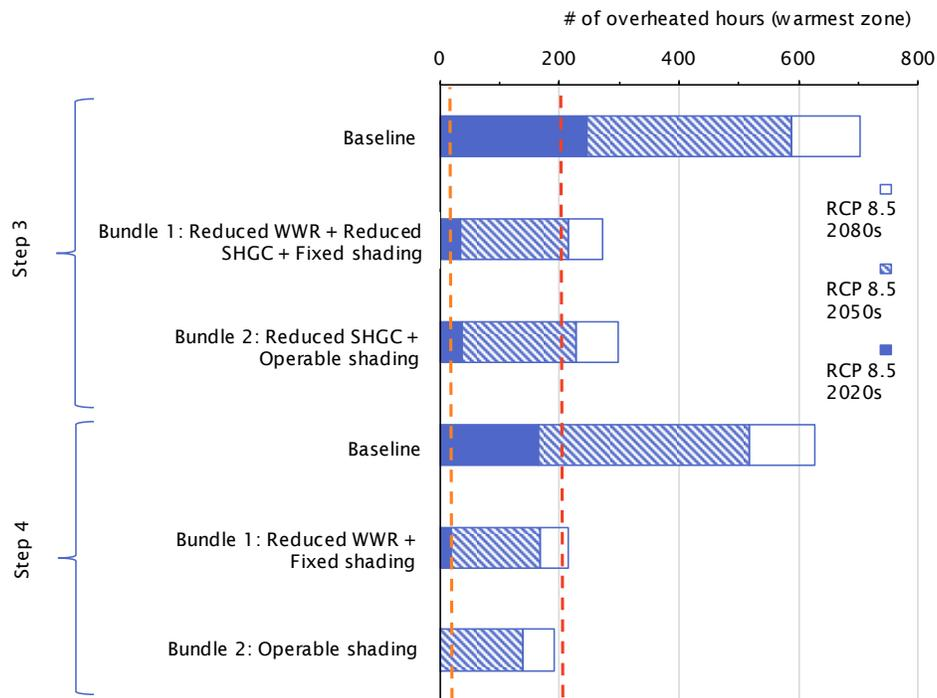
Figure 0.16 Number of overheated hours for the warmest zone, modelled with the RCP-8.5 2020s, 2050s, and 2080s climate files. The red dashed line illustrates the 200 hour threshold, and the orange dashed line illustrates the 20 hour threshold for vulnerable populations.
