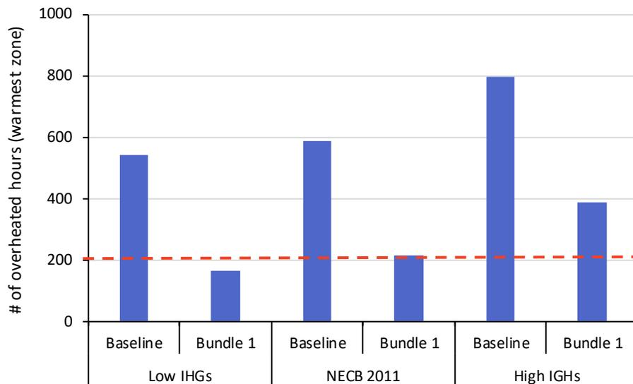
Figure 4.1 Sensitivity analysis of internal heat gains based on new building low rise archetype and Bundle 1, modelled with the RCP-8.5 2050s climate file.
