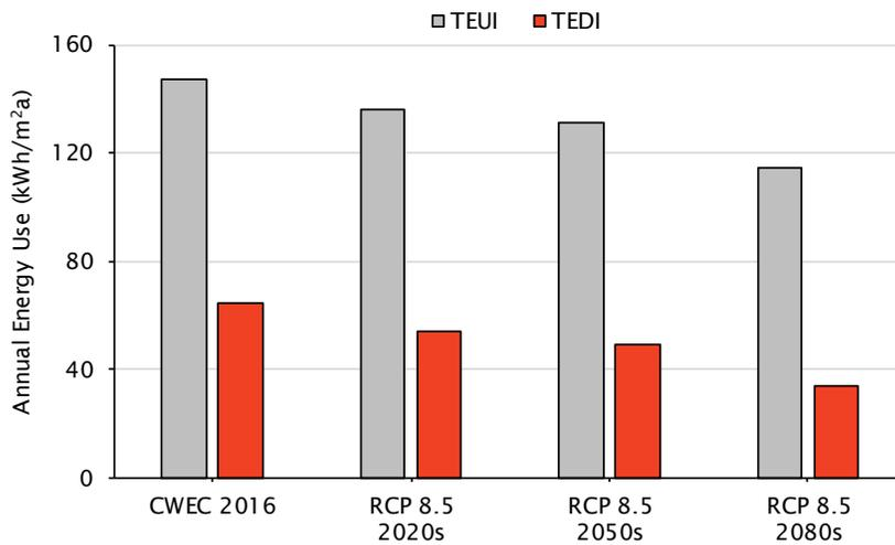
Figure 3.32 Annual total energy use intensity (TEUI) and thermal energy demand intensity (TEDI) results for the low rise existing building baseline.
