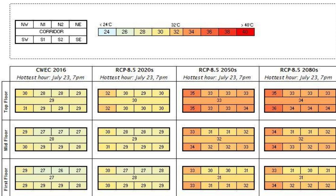
*Figure 3.2 Modelled peak operative temperature (°C) for each zone and climate file. The zones are colour coded to illustrate the variation in peak temperature.*
