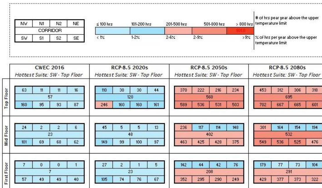
Figure 3.1 Number of hours that exceed the 80% acceptability limit. The zones that meet the 200 hr limit are shown as blue. The zones that exceed the 200 hr limit are colour coded as different shades of red. A darker red indicates a higher number of overheated hours.
