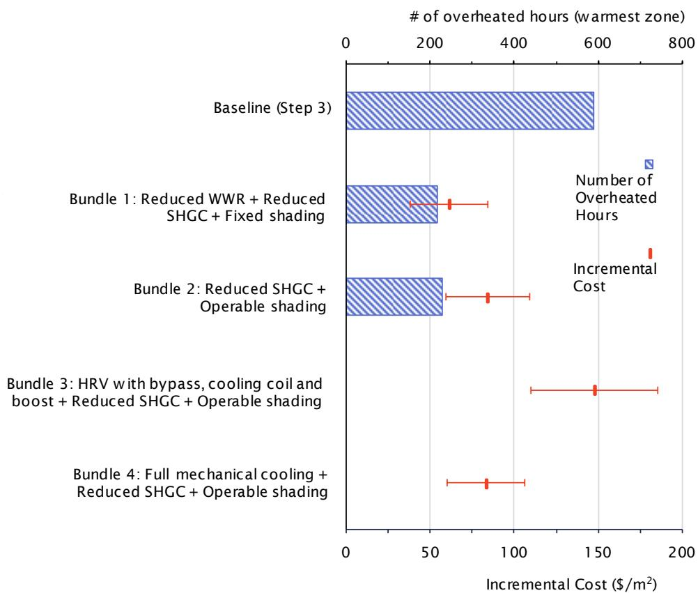
*Figure 3.9 Incremental cost (\$/m<sup>2</sup>) for the Step 3 bundles shown together with the number of overheated hours based on RCP-8.5 2050s climate file. The error bars show the high and low incremental bundle cost.*
