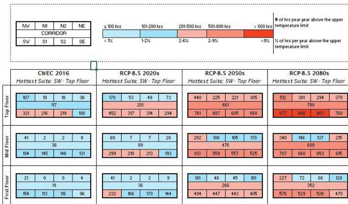
*Figure 3.29 Number of hours that exceed the 80% acceptability limit reported at zone level for each floor of the low rise existing building baseline. The zones that do not exceed the limit of 200 overheated hours are shown as blue. The zones that exceed the 200 hour limit are colour coded as different shades of red. A darker red indicates a higher number of overheated hours.*
