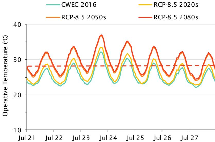
Figure 3.31 shows the modelled hourly operative temperature for the warmest suite during the warmest week for the low rise existing building baseline. The operative temperature is shown based on the CWEC 2016 climate file and RCP-8.5 2020s, 2050s and 2080s. The red dashed line illustrates the 80% acceptability limit based on the CWEC 2016 file.
