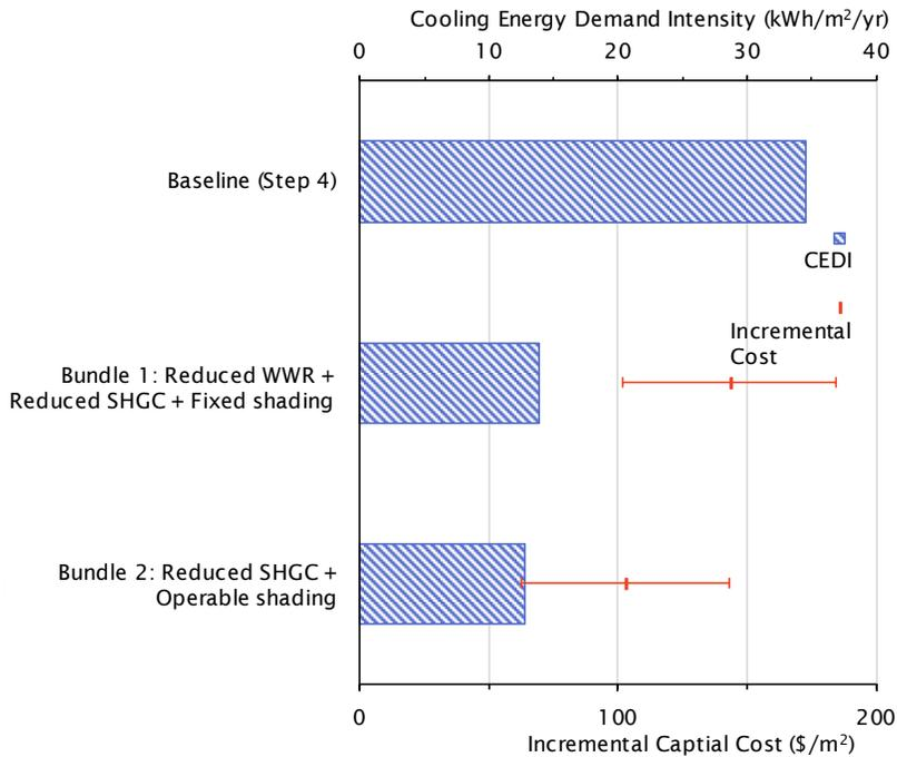
Figure 3.27 Incremental cost (\$/m<sup>2</sup>) for the Step 4 bundles shown together with the number of overheated hours based on RCP-8.5 2050s climate file. The error bars show the high and low incremental bundle cost.
