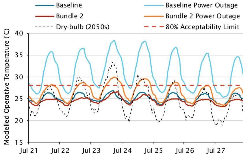
Figure 4.3 Modelled operative temperature for the Step 4 high rise new building baseline and Bundle 2, during normal operation and during a power outage event for a summer week.
