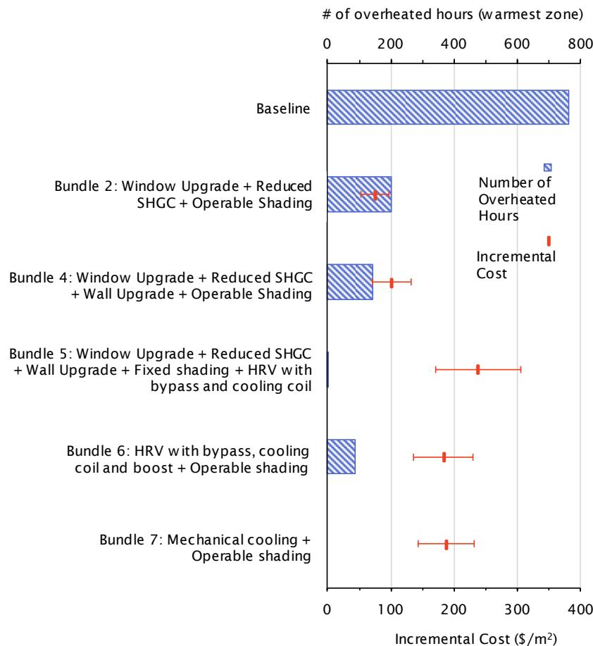
Figure 3.37 Incremental cost (\$/m<sup>2</sup>) for the bundles shown together with the number of overheated hours based on RCP-8.5 2050s climate file. The error bars show the high and low incremental bundle cost.
