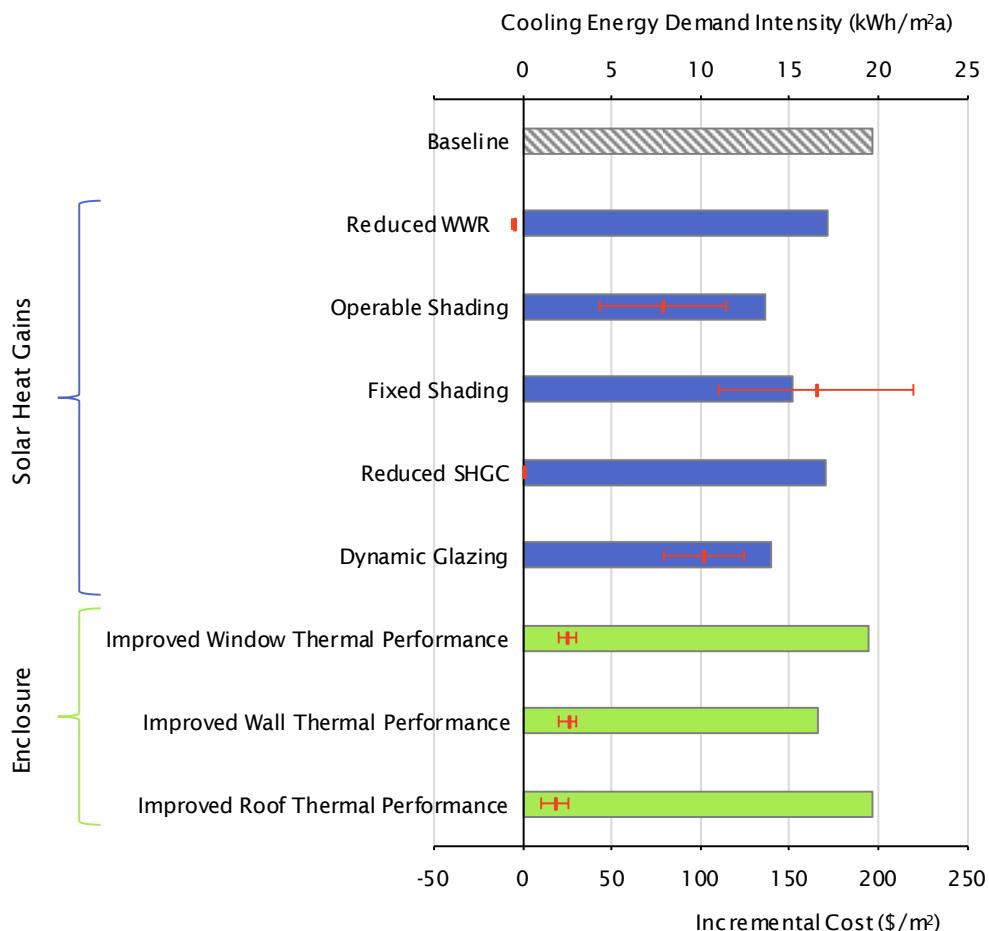
*Figure 3.19 The red lines show the incremental cost (\$/m<sup>2</sup>) on building level, the error bars show the high and low cost. The number of overheated hours is shown for the warmest suite based on RCP-8.5 2050s climate file*
