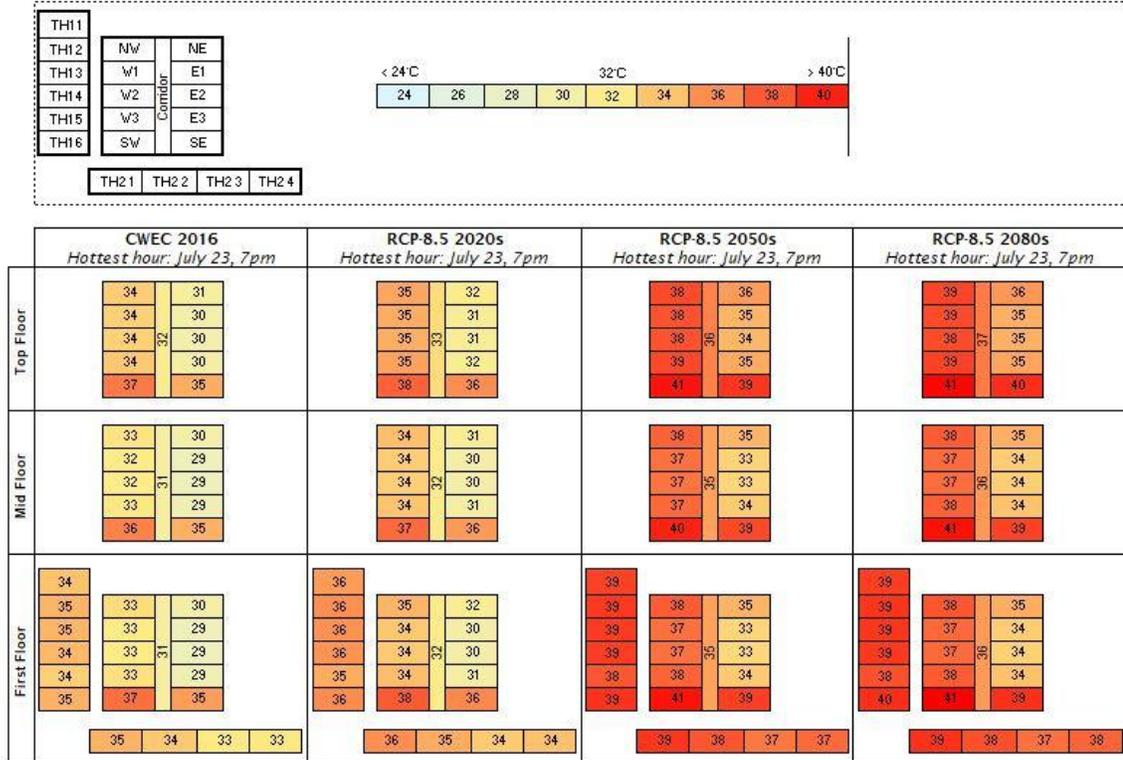
Figure 3.40 Modelled peak operative temperature (°C) for each suite and climate file. The zones are colour coded to illustrate the variation in peak operative temperature. A darker shade of red indicates a higher modelled peak temperature.
