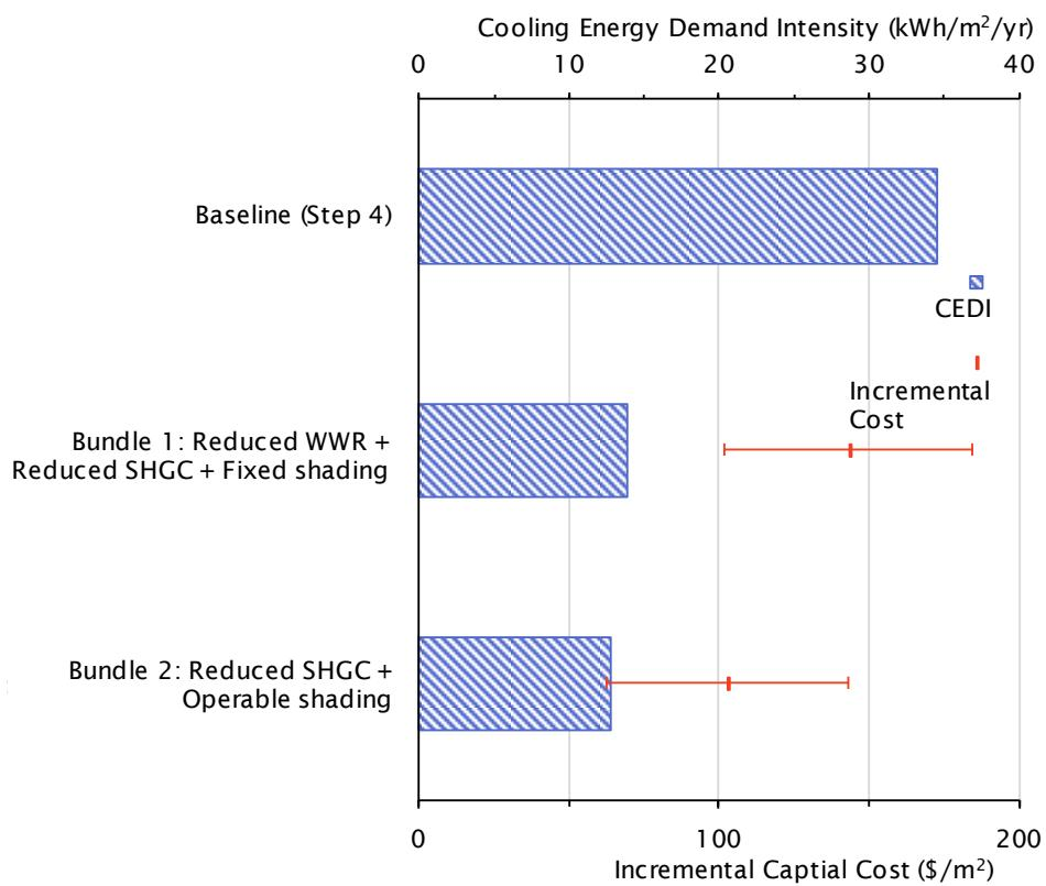
*Figure 0.6 Incremental cost (\$/m<sup>2</sup>) for the Step 4 high rise bundles shown together with the number of overheated hours based on RCP-8.5 2050s climate file. The error bars show the high and low incremental bundle cost.*
