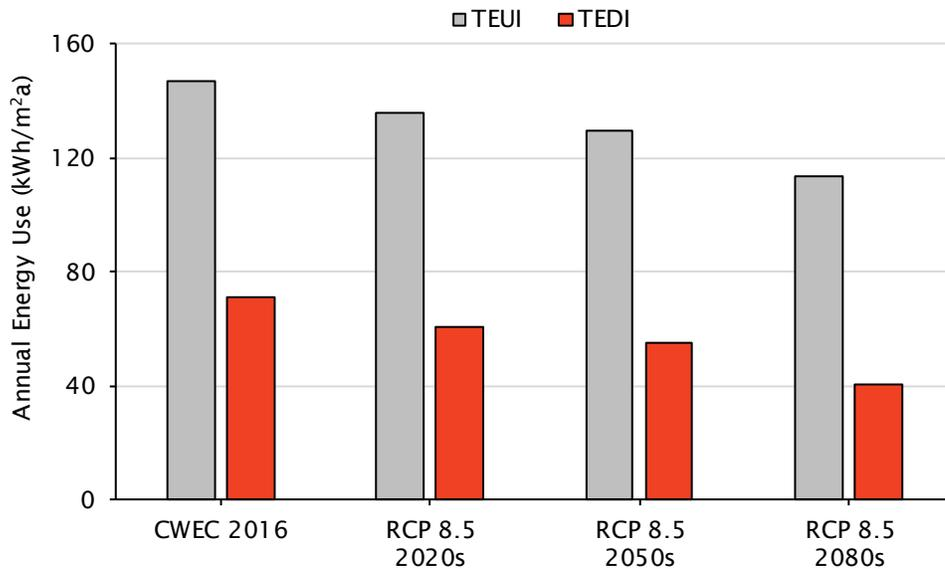
Figure 3.42 Annual total energy use intensity (TEUI) and thermal energy demand intensity (TEDI) results for the high rise existing building baseline.
