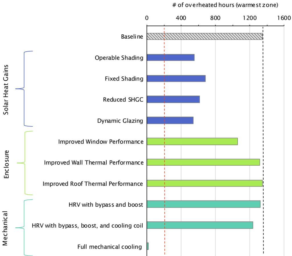
Figure 3.43 Number of overheated hours for the warmest suite and each individual climate adaptation measure, modelled with the RCP-8.5 2050s climate file. The red dashed line illustrates the 200 hour limit, and the black dashed line presents the baseline results.
