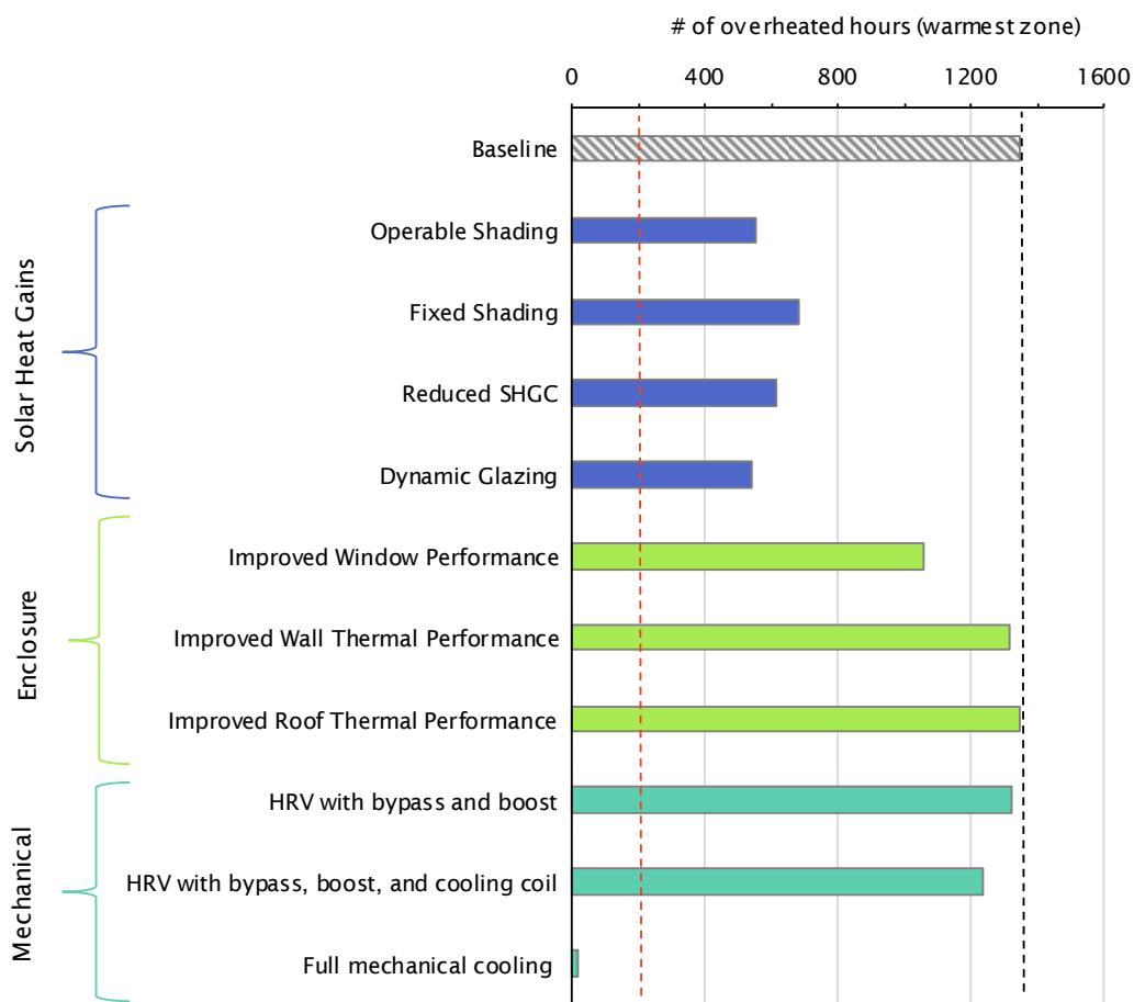
*Figure 3.43 Number of overheated hours for the warmest suite and each individual climate adaptation measure, modelled with the RCP-8.5 2050s climate file. The red dashed line illustrates the 200 hour limit, and the black dashed line presents the baseline results.*
