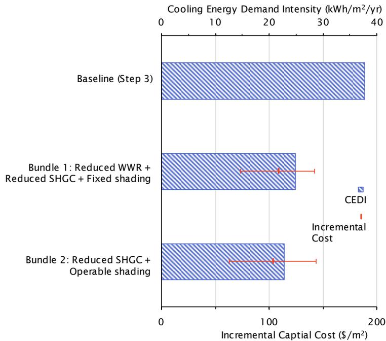
Figure 3.23 Incremental cost (\$/m<sup>2</sup>) for the Step 3 bundles shown together with the number of overheated hours based on RCP-8.5 2050s climate file. The error bars show the high and low incremental bundle cost.
