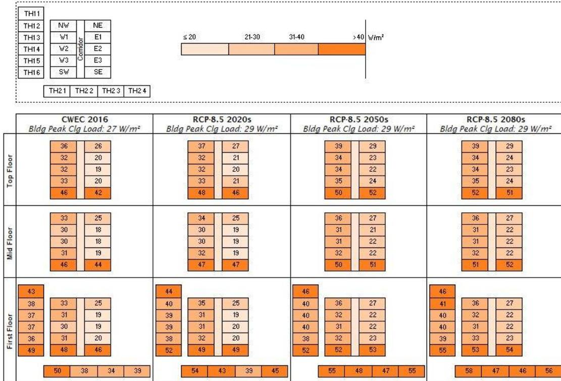
Figure 3.16 Peak cooling load (W/m<sup>2</sup>) at zone level for each climate scenario. A darker shade of orange indicates a higher peak cooling load. Note that the peak cooling load does not account for system efficiency.
