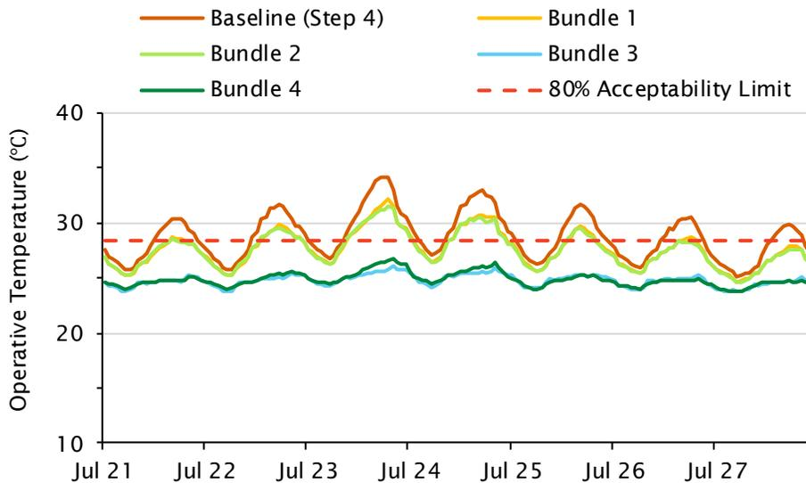
Figure 3.12 Modelled operative temperature (°C) for the warmest suite for the Step 4 low rise new building bundles, shown for the hottest summer week.
