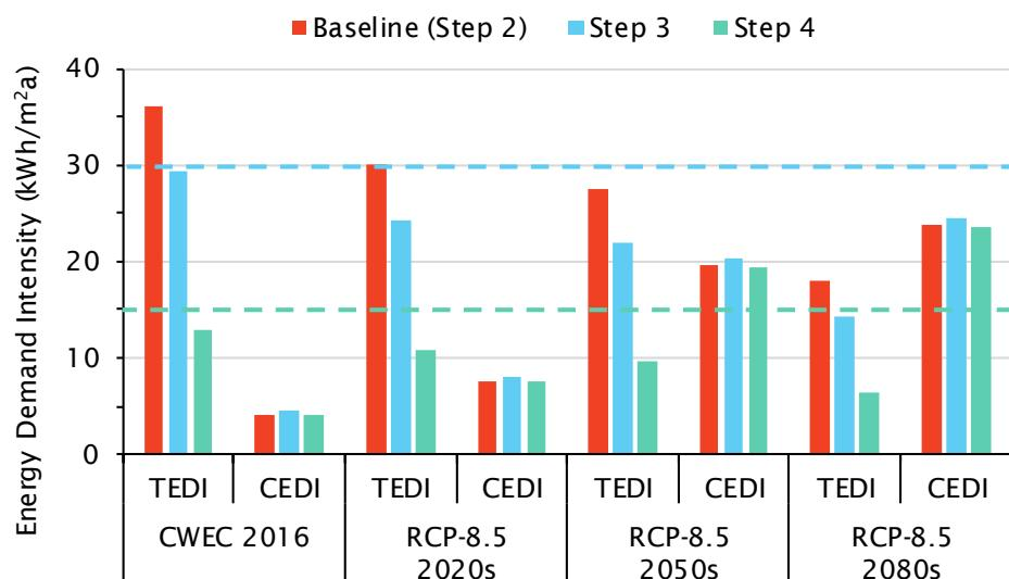
Figure 3.20 TEDI and CEDI for the baseline (Step 2) archetype and bundle baselines (Step 3 and Step 4), the blue and green dashed line show the TEDI target for Step 3 (30 kWh/m<sup>2</sup>a) and Step 4 (15 kWh/m<sup>2</sup>a), respectively.
