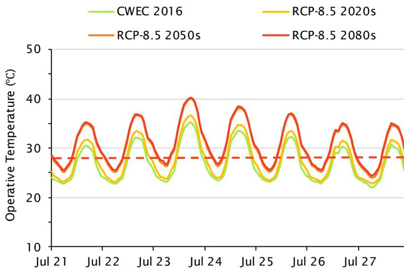
Figure 3.41 Modelled operative temperature (°C) for the warmest suite for the high rise existing building baseline. The interior temperature is shown for one summer week, based on the CWEC 2016, RCP-8.5 2020s, 2050s and 2080s climate files. The red dashed line illustrates the 80% acceptability limit based on the CWEC 2016 climate file.
