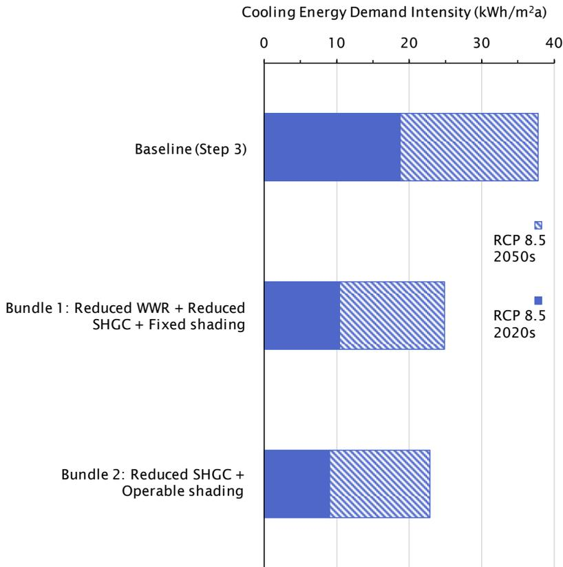
Figure 3.21 Cooling energy demand intensity (kWh/m²a) for the warmest suite for the Step 3 baseline and modelled bundles, for RCP-8.5 2020s and 2050s climate files.
