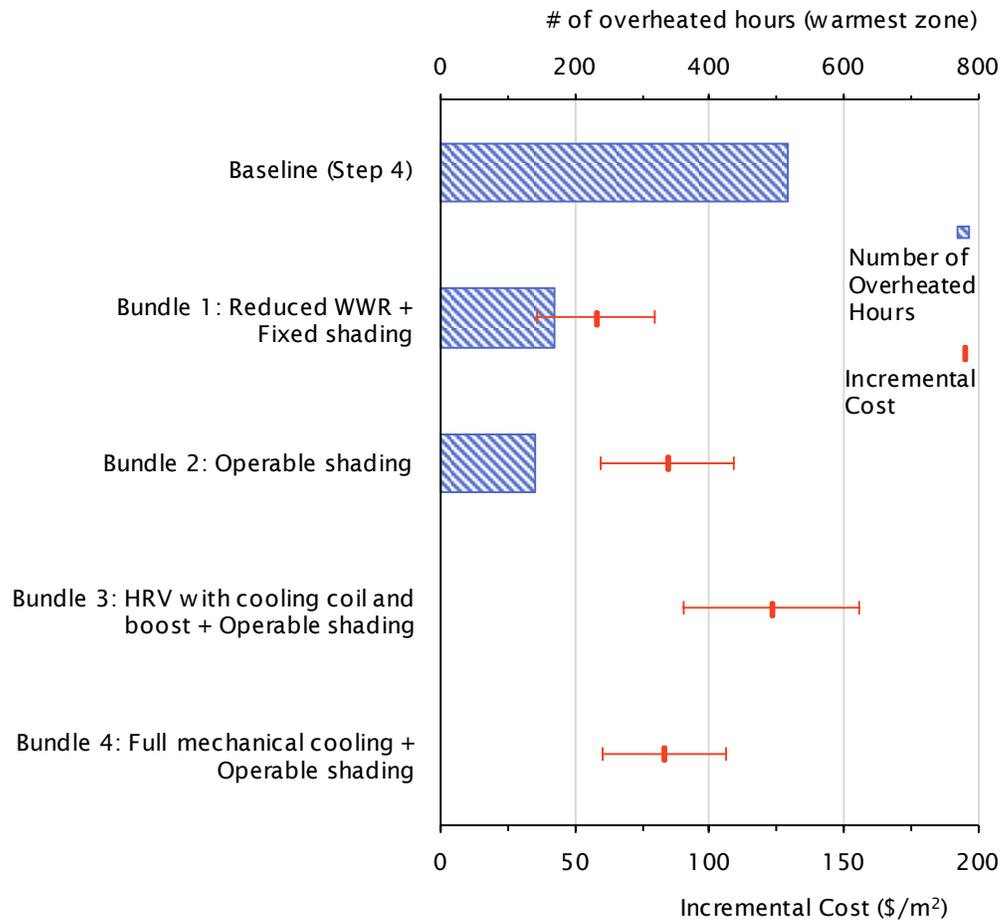
Figure 3.13 Incremental cost (\$/m<sup>2</sup>) for the Step 4 bundles shown together with the number of overheated hours based on RCP-8.5 2050s climate file. The error bars show the high and low incremental bundle cost.
