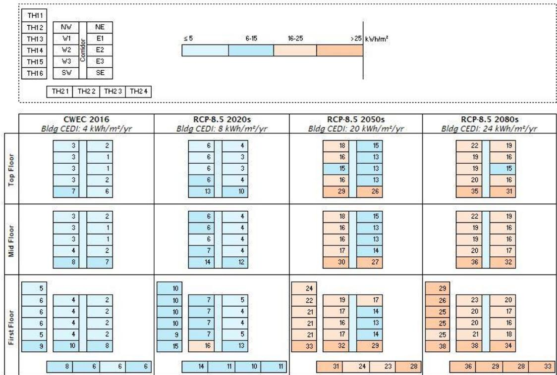
Figure 3.15 Cooling energy demand intensity (kWh/m<sup>2</sup>a) at zone level for each climate file. The zones that have a CEDI lower than the Passive House Institute requirement (15 kWh/m<sup>2</sup>a) are shown as blue. The zones that exceed 15 kWh/m<sup>2</sup>a are colour coded in different shades of orange. A darker orange indicates a higher CEDI.
