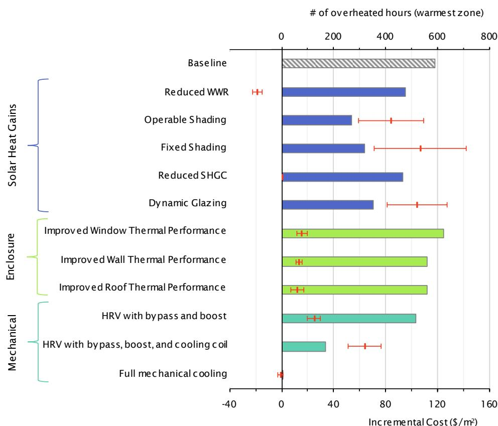
*Figure 3.6 The red lines show the incremental cost (\$/m<sup>2</sup>) on building level, the error bars show the high and low cost. The number of overheated hours is shown for the warmest suite based on RCP-8.5 2050s climate file.*
