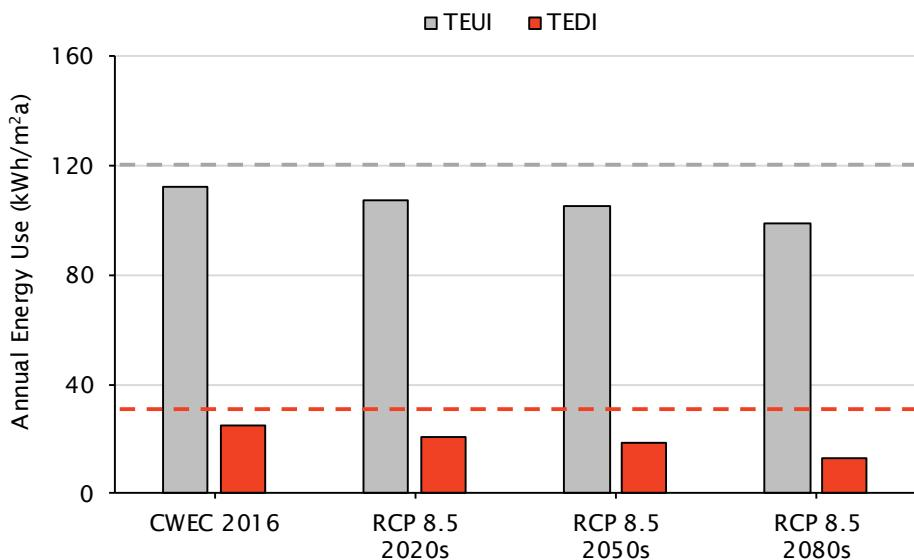
*Figure 3.4 Annual total energy use intensity (TEUI) and thermal energy demand intensity (TEDI) results for the low rise new building baseline. The grey dashed line shows the Step 3 TEUI target (120 kWh/m<sup>2</sup>a), and the red dashed line shows the Step 3 TEDI target (30 kWh/m<sup>2</sup>a).*
