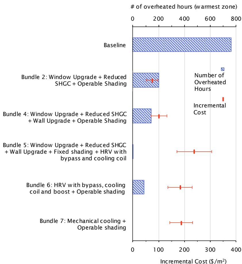
*Figure 0.9 Incremental cost (\$/m<sup>2</sup>) for the bundles shown together with the number of overheated hours based on RCP-8.5 2050s climate file. The error bars show the high and low incremental bundle cost.*
