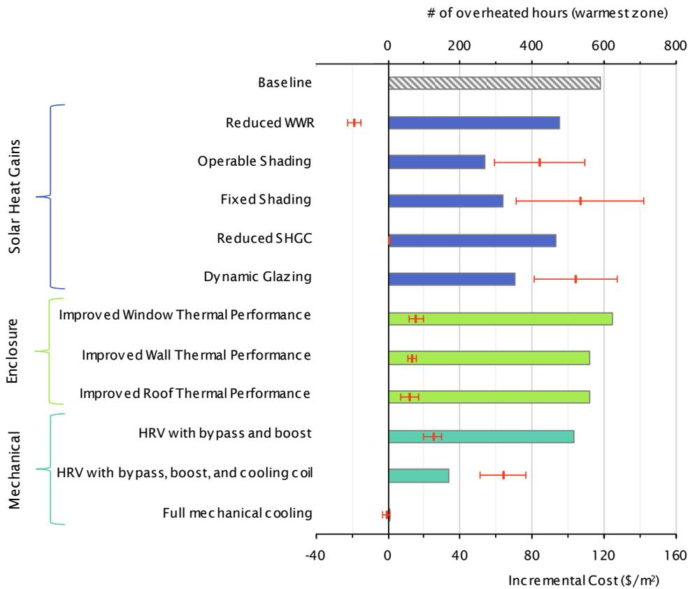
Figure 3.6 The red lines show the incremental cost (\$/m²) on building level, the error bars show the high and low cost. The number of overheated hours is shown for the warmest suite based on RCP-8.5 2050s climate file.
