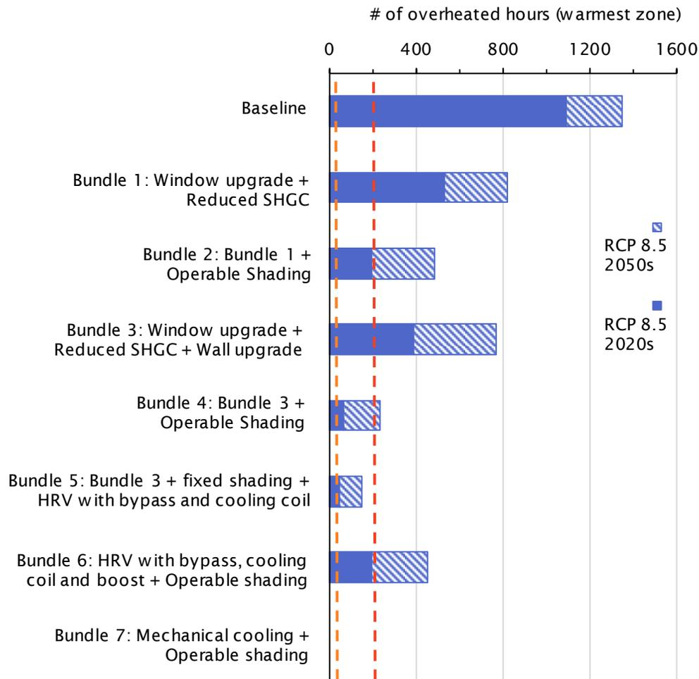
Figure 3.45 Number of overheated hours for the warmest suite for each modelled bundle. The red dashed line illustrates the 200 hour limit, the orange dashed line illustrates the 20 hour limit for vulnerable population.
