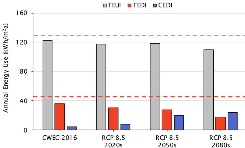
Figure 3.17 Annual total energy use intensity (TEUI), thermal energy demand intensity (TEDI) results and cooling energy demand intensity (CEDI) for the high rise new building baseline. The grey dashed line shows the Step 2 TEUI target (130 kWh/m<sup>2</sup>a), and the red dashed line shows the Step 2 TEDI target (45 kWh/m<sup>2</sup>a).
