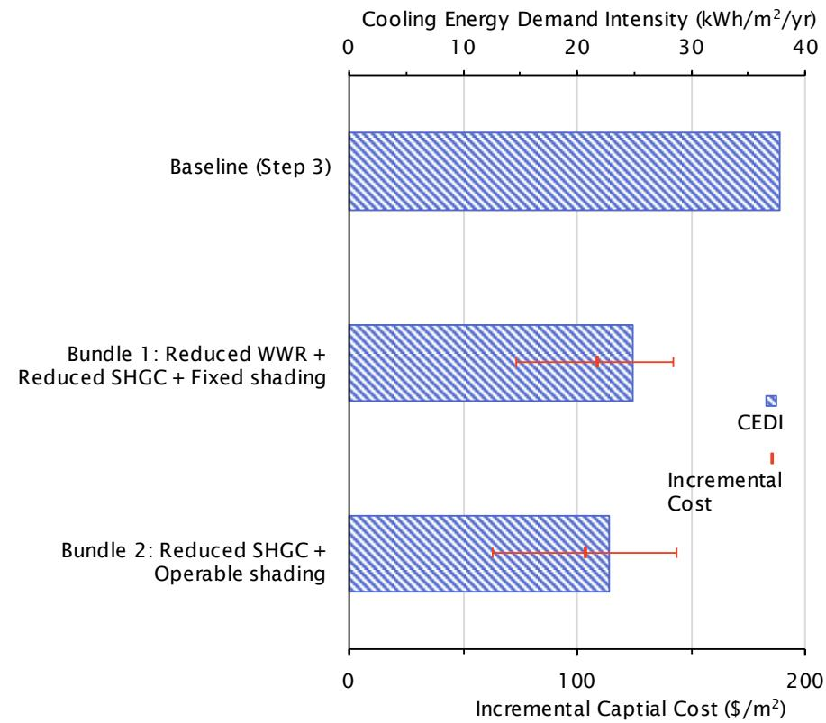
*Figure 0.5 Incremental cost (\$/m<sup>2</sup>) for the Step 3 high rise bundles shown together with the number of overheated hours based on RCP-8.5 2050s climate file. The error bars show the high and low incremental bundle cost.*
