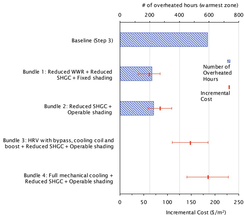
*Figure D.1 Incremental cost (\$/m<sup>2</sup>) for the Step 3 bundles shown together with the number of overheated hours based on RCP-8.5 2050s climate file. The error bars show the high and low incremental bundle cost.*
