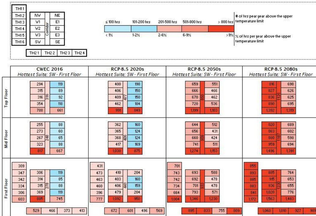
Figure 3.39 Number of hours that exceed the 80% acceptability limit reported at suite level for representative floors of the high rise existing building baseline. The suites that do not exceed the limit of 200 overheated hours are shown as blue, and the suites that exceed the 200-hour limit are colour coded as different shades of red, a darker shade of red indicate a higher number of overheated hours.
