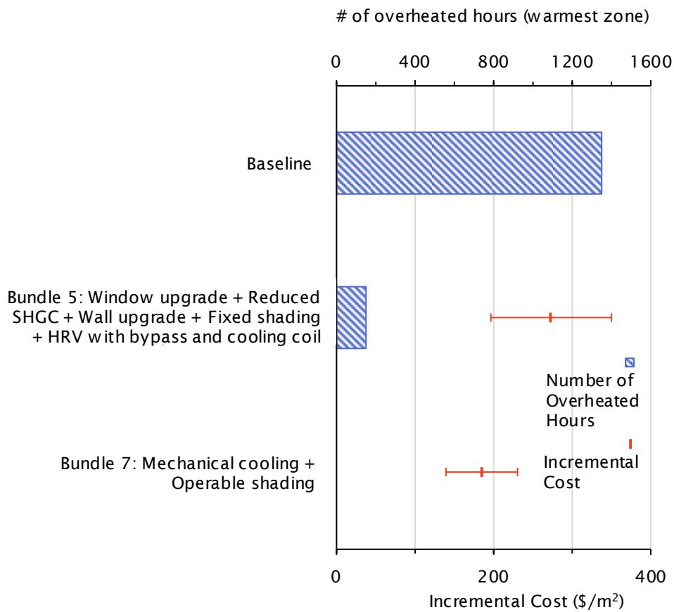
*Figure 0.11 Incremental cost (\$/m<sup>2</sup>) for the bundles shown together with the number of overheated hours based on RCP-8.5 2050s climate file. The error bars show the high and low incremental bundle cost.*
